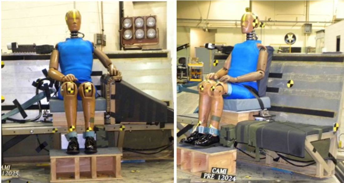
Figure 3: Lap Belt-Only Test Setup: Armrest (left) and No Wall (right)
