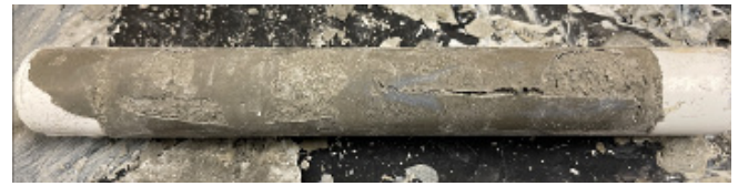
Figure 5. Photo. An encapsulated specimen wrapped in poor-quality grout.
