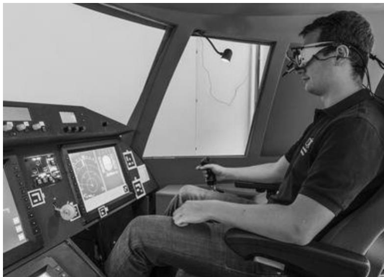
Figure 11. Eyetracking glasses in use in a simulator (from Haslbeck and Bengler 2016)
