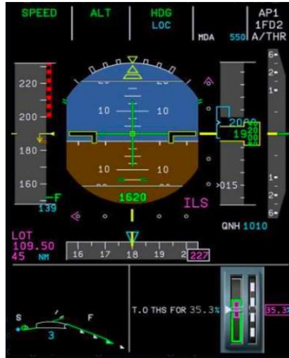
Figure 27. Airbus A350 Primary Flight Display (PFD) with flap and thrust lever settings (bottom left and bottom right of the PFD, respectively; from https://karlenepetitt.blogspot.com/2020/10/power-of-a350.html )
