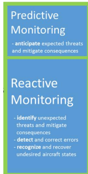
Figure 26. Two complementary forms of monitoring (image adopted from International Air Transport Association (IATA), 2016, page 21)
