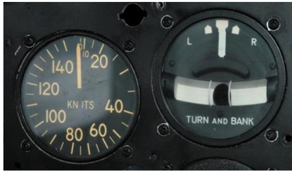
Figure 3. Airspeed (on the left) and turn-and-bank indicator (on the right) (from https://www.aircraftspruce.com/catalog/graphics/1/10-22614.jpg )
