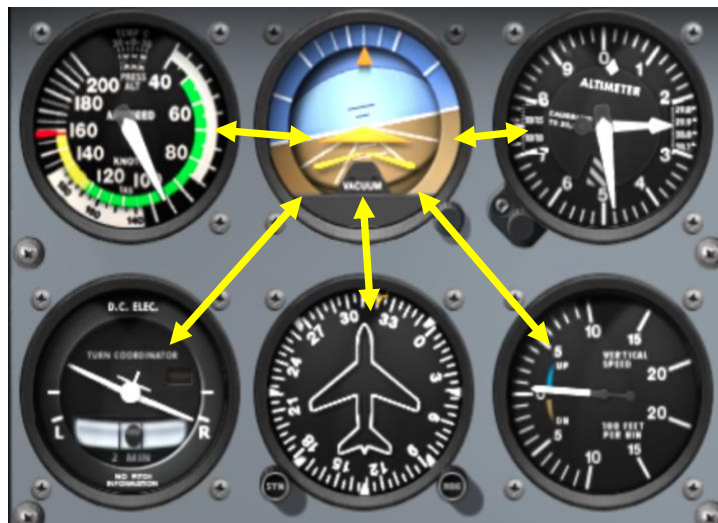
Figure 24. Radial scan pattern where the pilot spends most of the time looking at the attitude indicator, with quick glances at other instruments before returning to the attitude indicator (adapted from https://nashvillecfi.com/instrument/ils.cgi )
