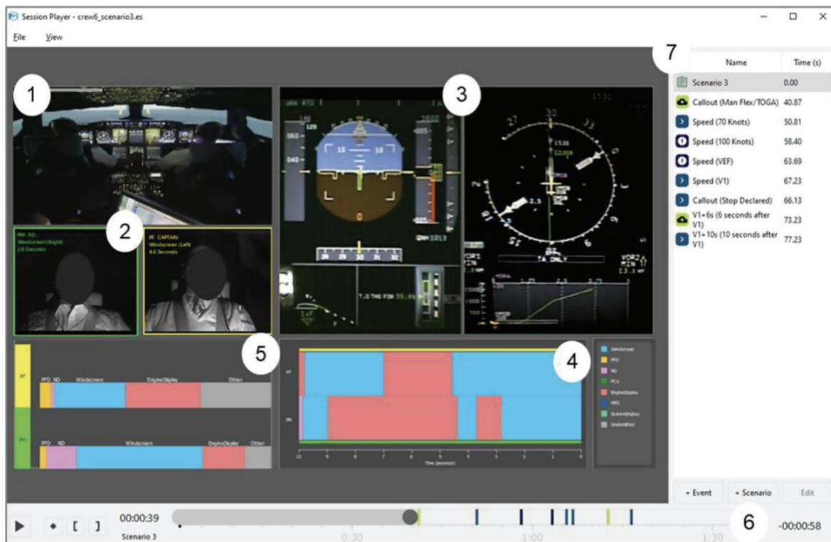
Figure 5. Prototype of the instructor interface (Session Player) components. (1) Cockpit view. (2) Face view. (3) Primary flight display (PFD) and navigation display (ND) overlaid with precise gaze vector and gaze trail presenting the real-time eye movements. (4) CandyBar. (5) Cumulative dwell time: A time plot illustrating dwell time over elapsed scenario/event time. (6) Start/stop bar and elapsed time axis. (7) Selectable event markers.
