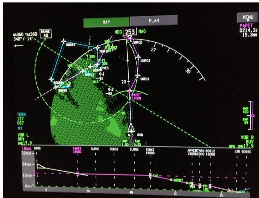
Figure 30: Sample view of the B 787 VSD (shown at the bottom of the PFD) (from https://twitter.com/peytour13/status/1054951808840425473/photo/1 )
