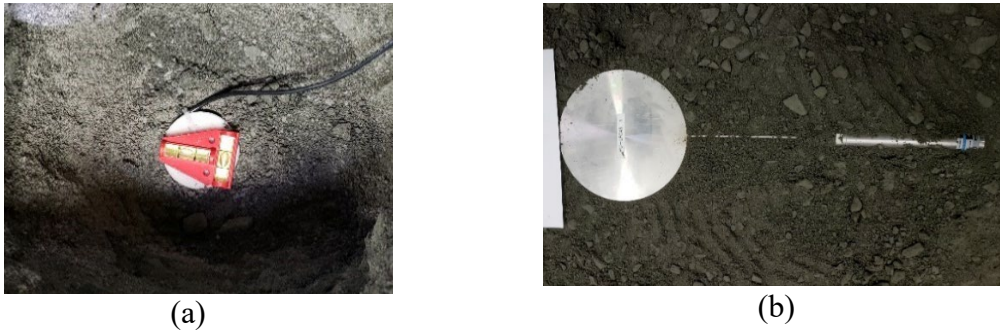
Figure 41. Embedded Sensors at NAPTF CC9: (a) Inductive CS Pairs and (b) PC
