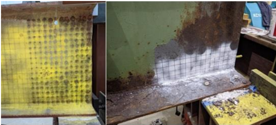
Figure 3.1: Point measurement grids for PocketMIKE (67) ultrasonic thickness gauge
