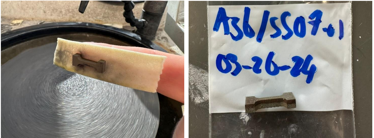
Figure 2-21: Tensile coupon obtained with EDM
