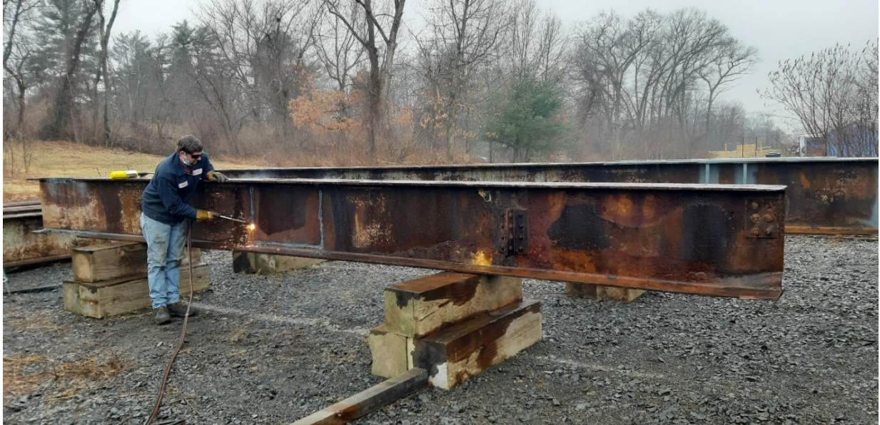
Figure 2-1: Steel plate extraction from A36 beam element
