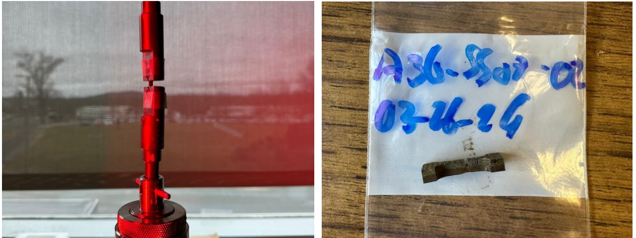
Figure 2-22: Testing rig tension coupons and end result of a composite coupon
