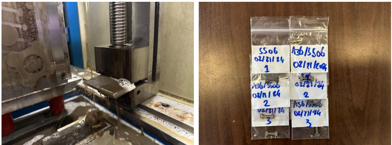
Figure 2-20: Final cutting and tensile coupons obtained with EDM
