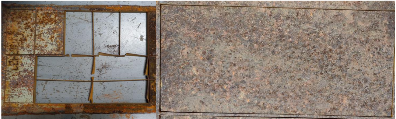
Figure 2-2: Steel specimen extraction by laser cutting
