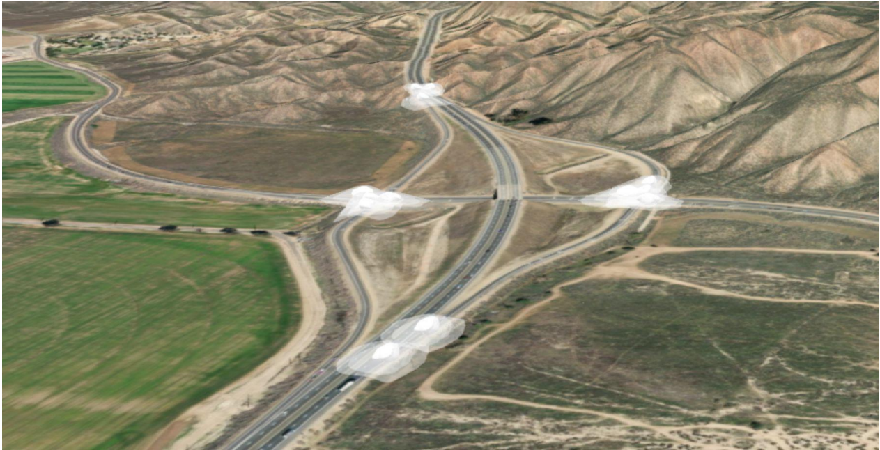
Figure 41. Three-dimensional visualization of 0.1, 1, and 10 lux (horizontal) light volumes for SR-79 and Gilman Springs Road, calculated native in a specialized GIS environment by EvariLux.
