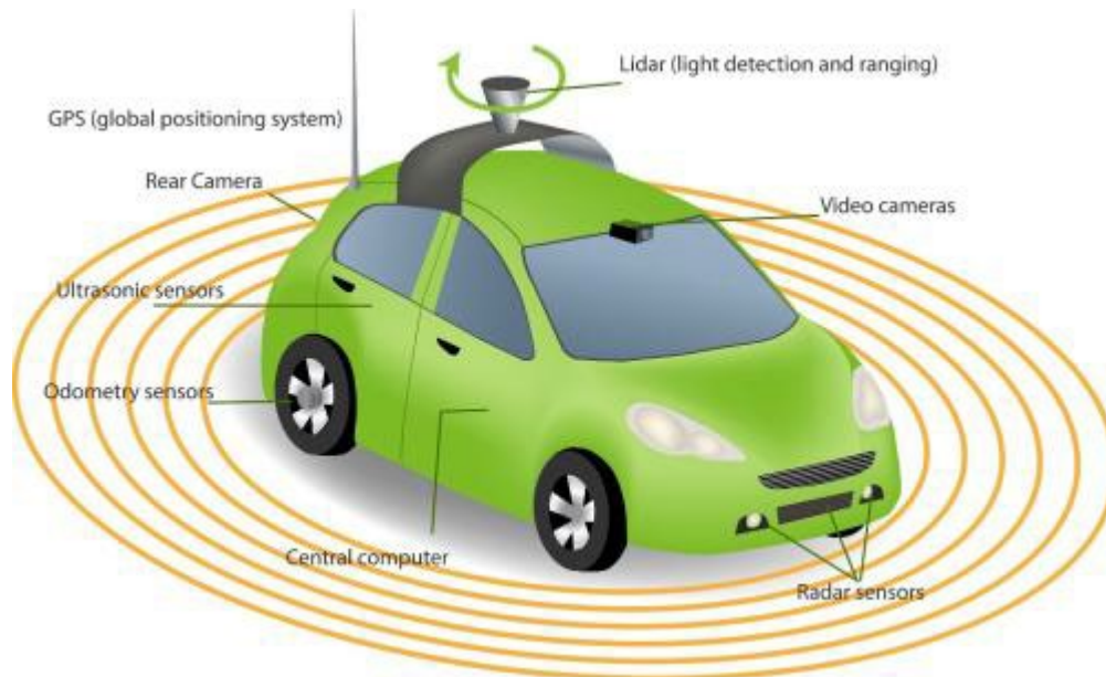
Figure 1: Automated Vehicle Sensors https://innovationnetwork.ieee.org/lidr-is-the-latest-game-changing-advancement-for-autonomous-vehicles/
