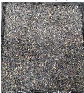
Figure 2: Slab with Epoxy and asphalt-based binder after 140K polishing cycles, Three-Wheel Polishing Device.
