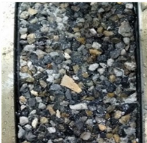
Figure 1: Calcined Bauxite HFST size with Emulsion (CRS-2P), British Pendulum coupons.
