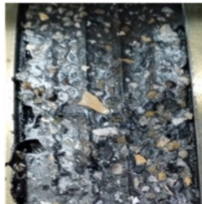
Figure 1: Calcined Bauxite HFST size with Emulsion (CRS-2P), British Pendulum coupons.
