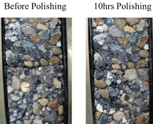
Figure C.2 Coupons with PG binders before and after polishing
