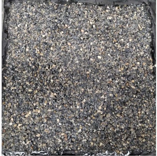
Figure C.7 Slabs with Epoxy resin (Left, CB/HFST. Right, CB/coarse)
