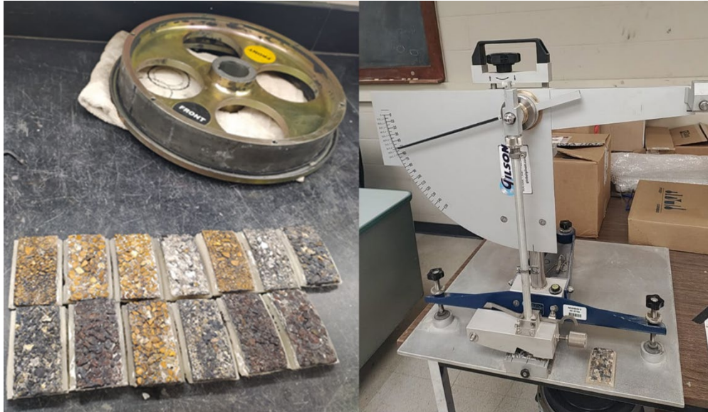
Figure B.2 BPT and PSV test placement
