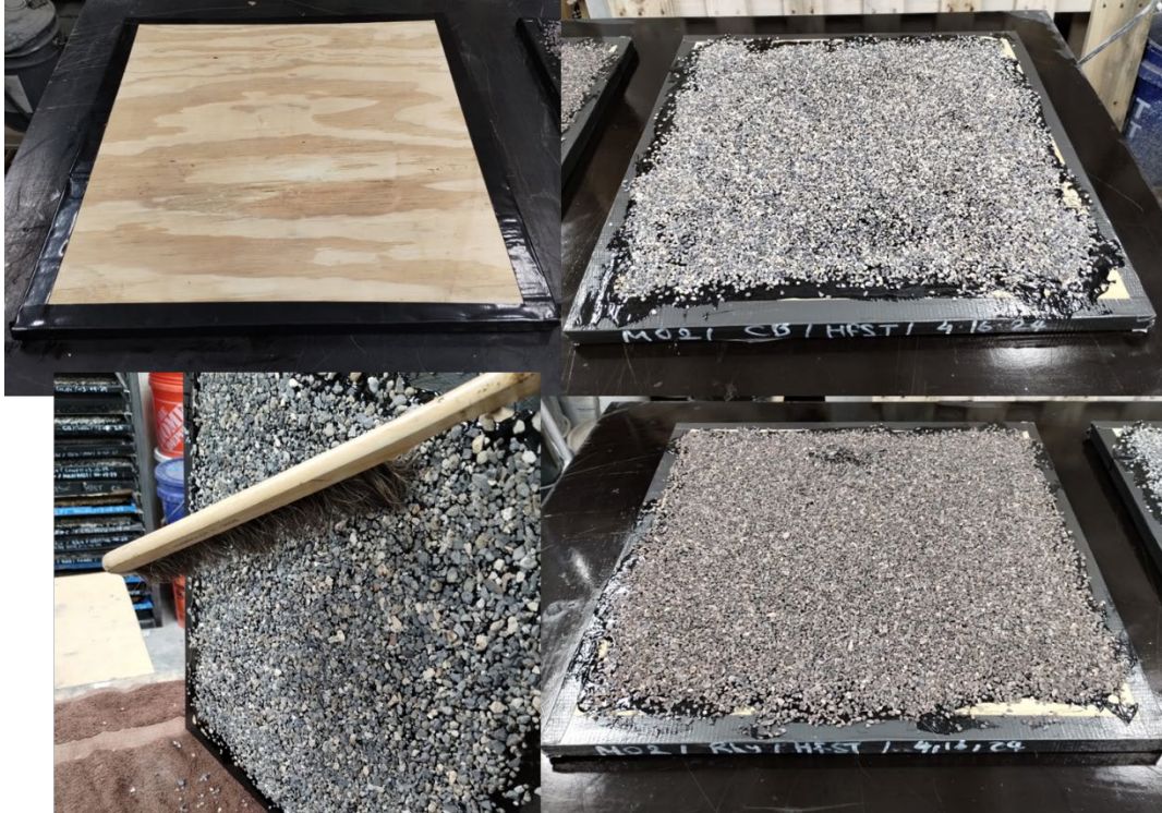
Figure B.4 Slab preparation with PG and modified asphalt binder
