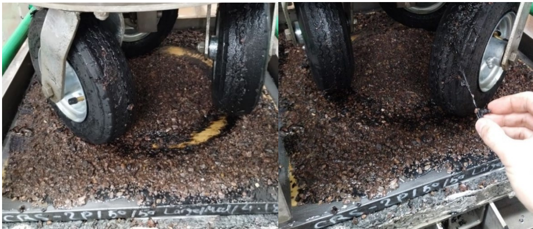
Figure 7.15 Severe bleeding and rutting in emulsion CRS-2P slab with new gradation after 30K polishing cycles
