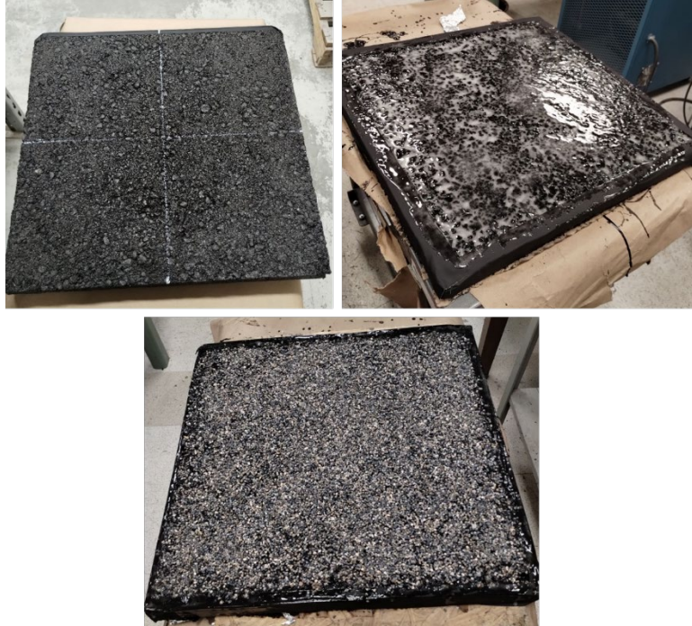
Figure B.3 Slab preparation with epoxy resin
