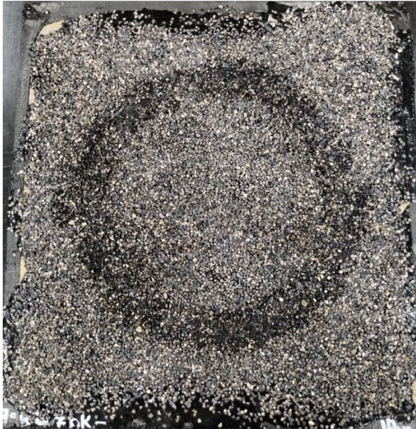
Figure C.9 Slabs with PG82-22(PM) (Left, CB/HFST. Right, CB/coarse)
