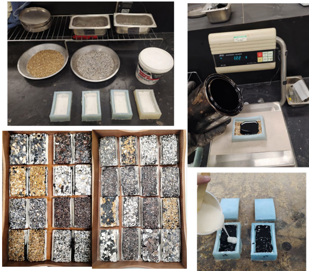
Figure B.1 The preparation process for the aggregate coupons
