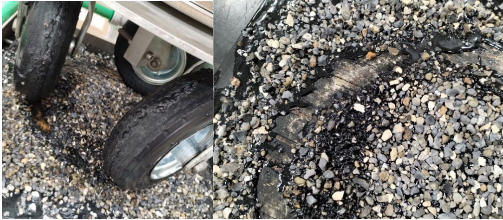
Figure 7.14 Severe bleeding and rutting in emulsion CRS-2P slab after 30K polishing cycles
