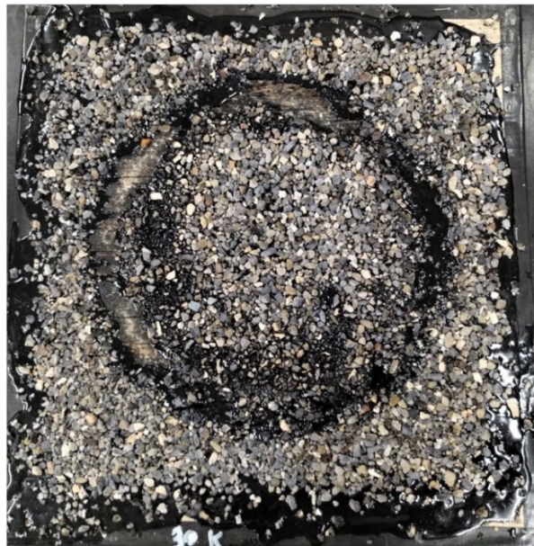
Figure C.12 Slabs with CRS-2P (Left, CB/HFST. Right, CB/coarse)
