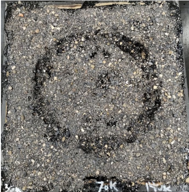
Figure C.11 Slabs with (Left, PG82-22(PM)/CB/medium. Right, PG88-16(PM)/CB/medium)
