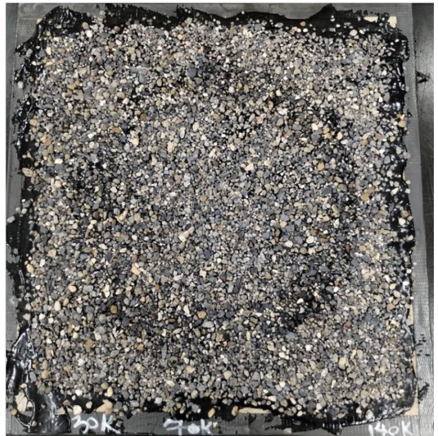
Figure C.10 Slabs with PG88-16(PM) (Left, CB/HFST. Right, CB/coarse)
