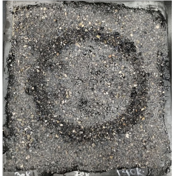
Figure C.11 Slabs with (Left, PG82-22(PM)/CB/medium. Right, PG88-16(PM)/CB/medium)
