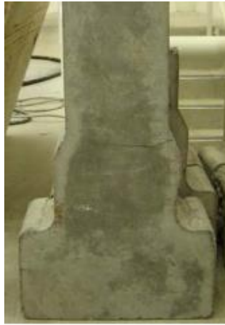
Figure 5-2: Double dog-bone geometry of a Uniaxial Direct Tensile test specimen (Chao et al., 2011)
