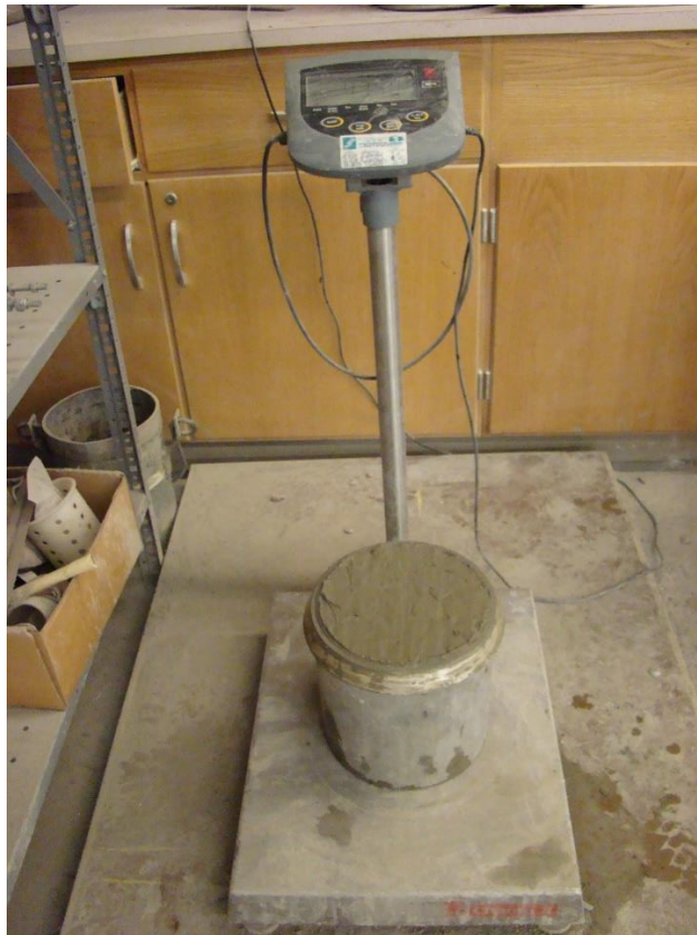
Figure 8-17: Determination of the fresh concrete unit weight, according to ASTM C138
