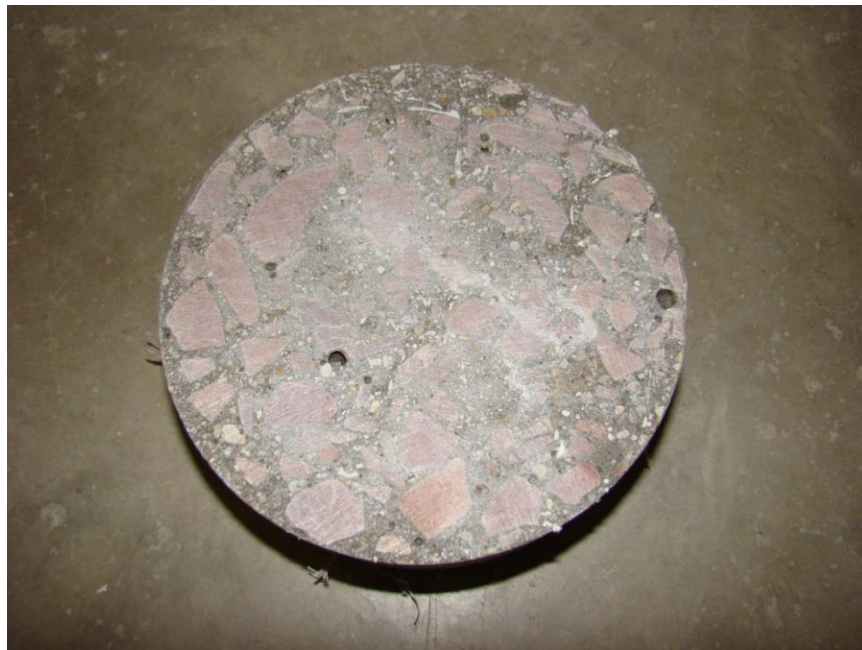
Figure 9-24: Cut surface of a synthetic FRC specimen
