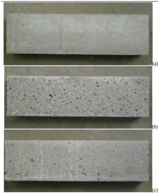
Figure 5-3: Surfaces of freeze-thaw specimens (a) before, (b) plain concrete after and (c) HyFRC after freeze-thaw cycling (Ostertag and Blunt, 2008)
