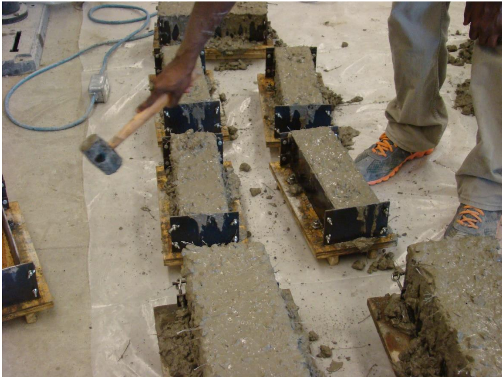
Figure 8-11: Use of rubber mallet to obtain final consolidation efforts of the concrete
