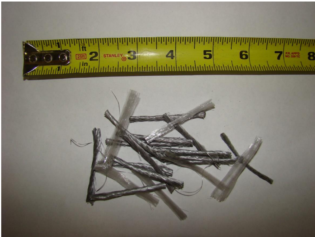
Figure 8-4: FORTA-FERRO fibers, manufactured by Forta Corporation
