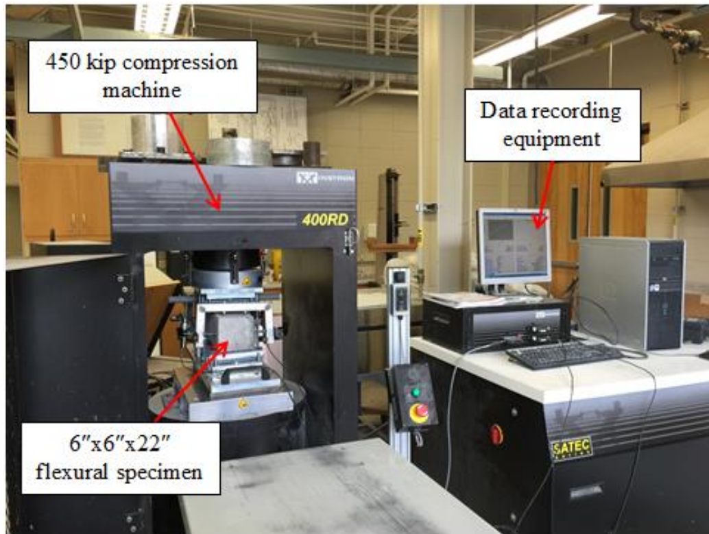
Figure 8-20: Flexural Performance (ASTM C1609) testing setup
