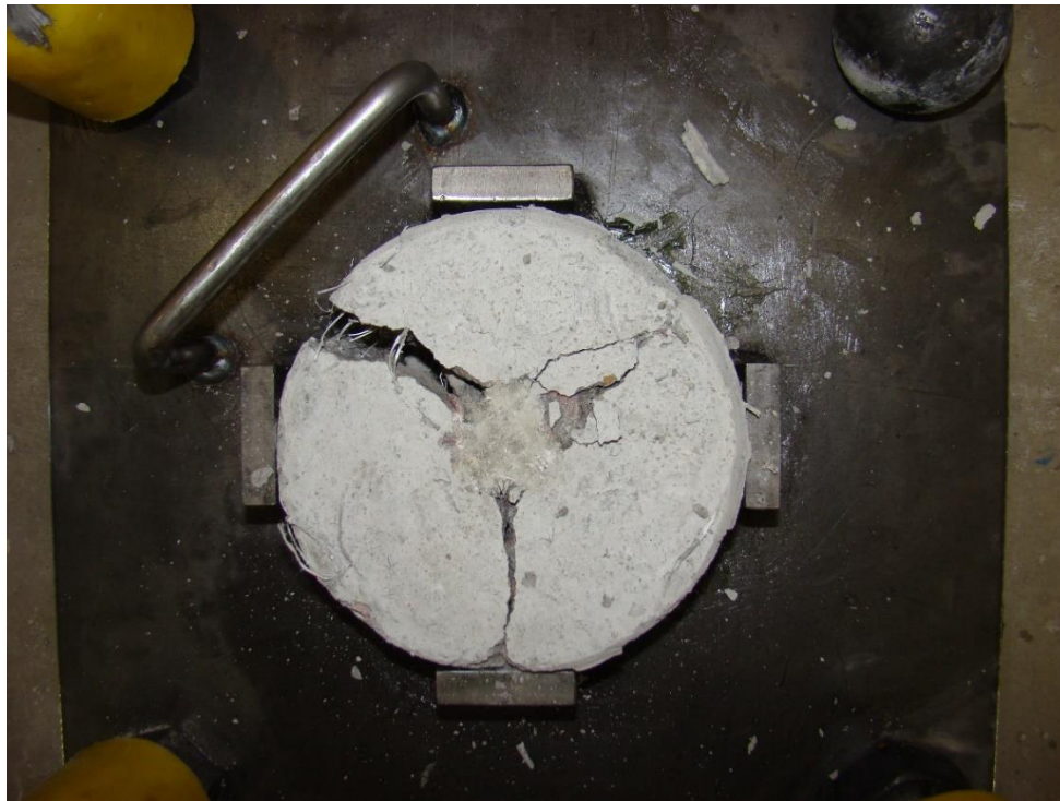
Figure 8-25: Failed impact specimen
