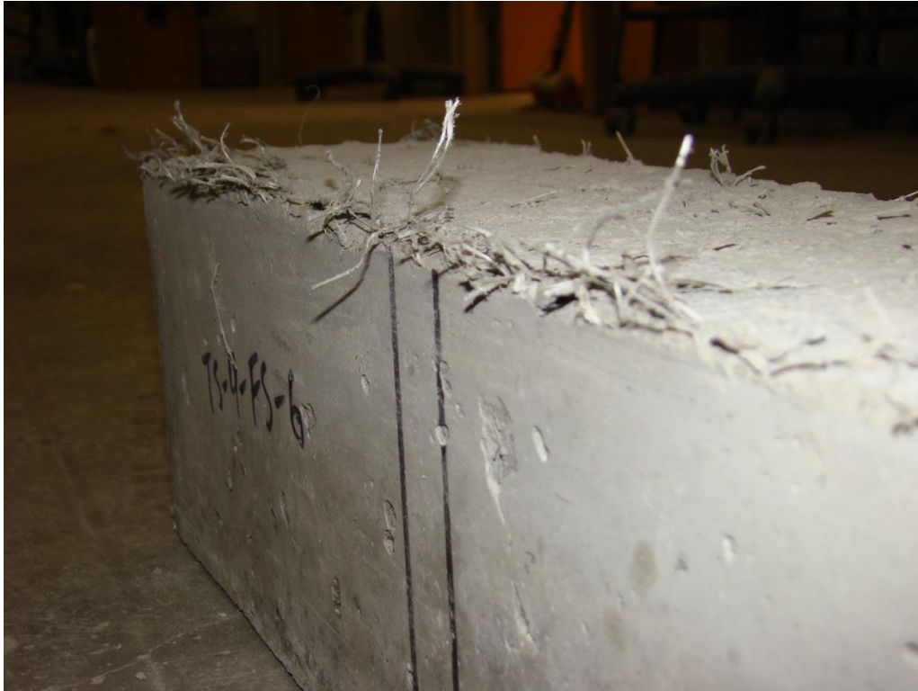
Figure 9-26: Hairy finished surface of a synthetic FRC specimen
