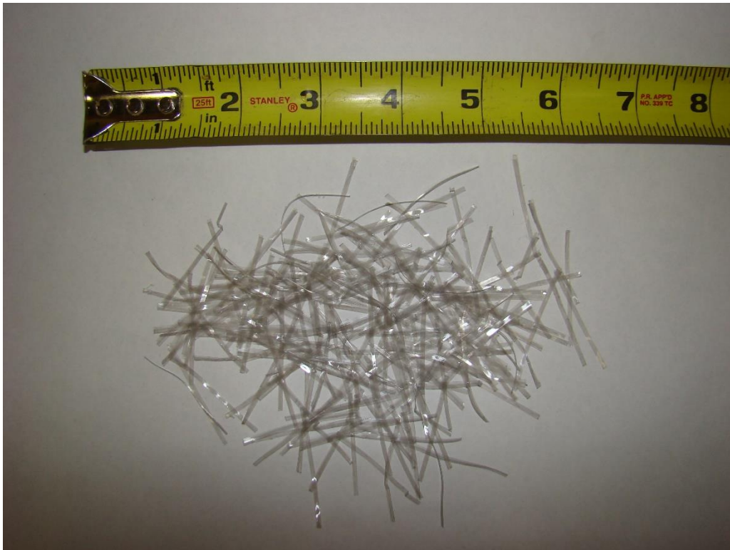
Figure 8-1: Strux 90/40 fibers, manufactured by W.R. Grace
