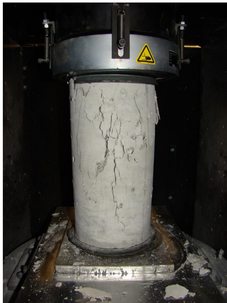
Figure 9-4: FRC compressive strength cylinder at failure
