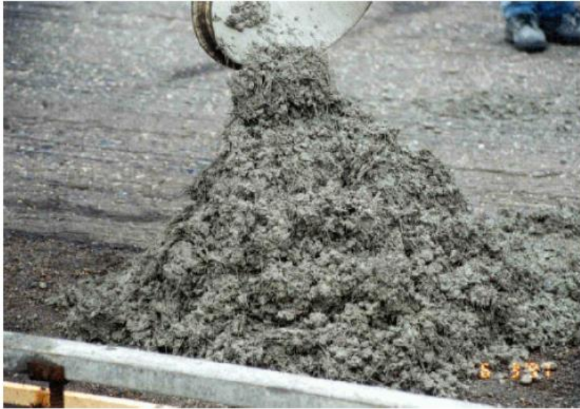
Figure 5-5: Consistency of a polyolefin FRC mix as it is discharged from the mixing truck (Dunn and Wolf, 2001)
