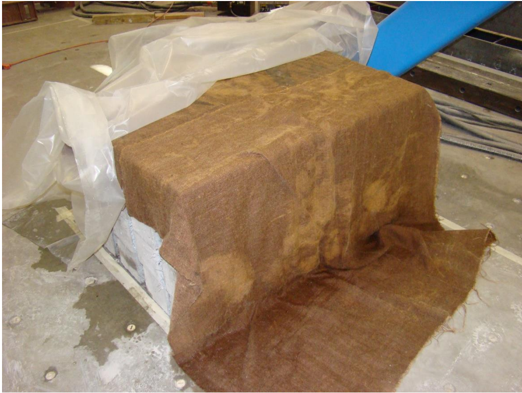
Figure 8-13: Wet burlap placed over the top of the concrete specimens in the curing chamber
