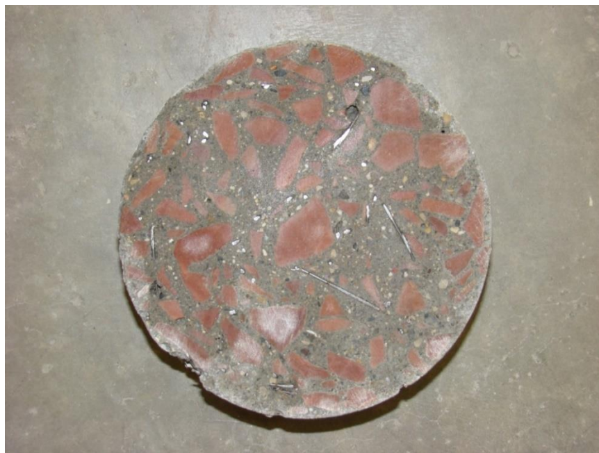
Figure 9-25: Cut surface of a steel FRC specimen
