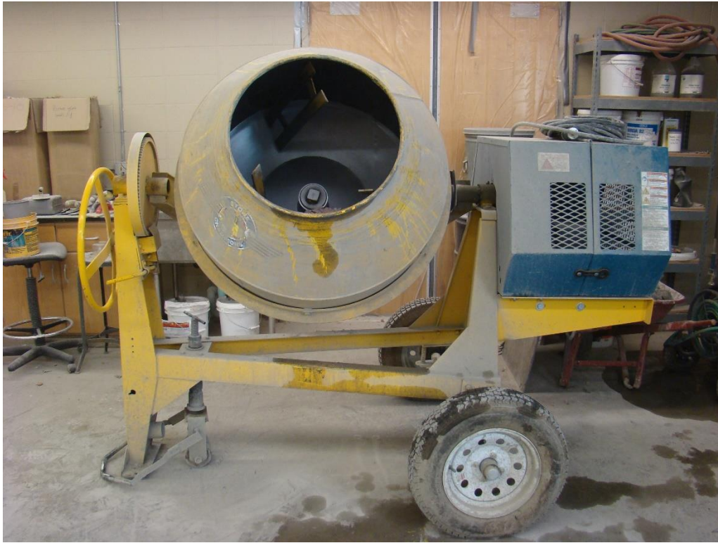
Figure 8-7: 1/2 cubic yard capacity concrete drum mixer
