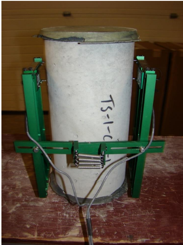
Figure 8-18: 8" Extensometer used to measure the compressive strain of a concrete cylinder during testing, according to ASTM C39
