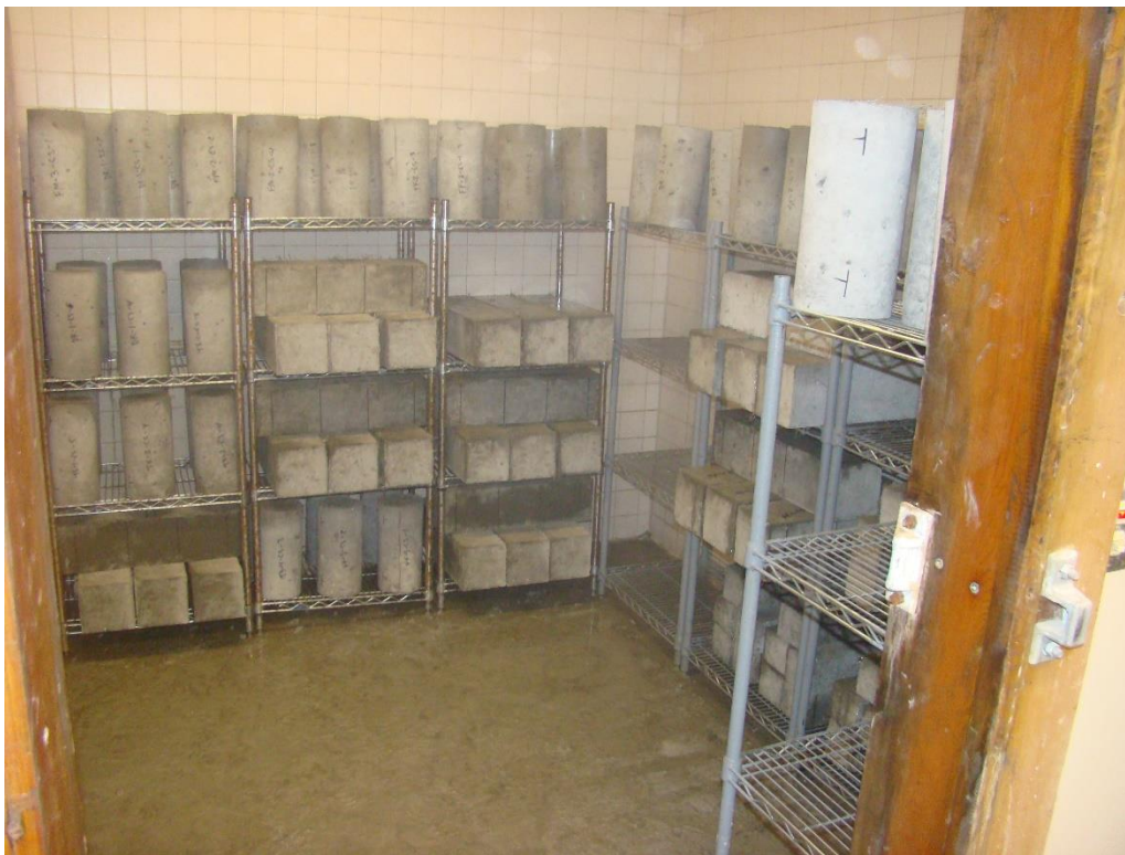
Figure 8-12: Moist cure room used to cure a majority of the testing specimens
