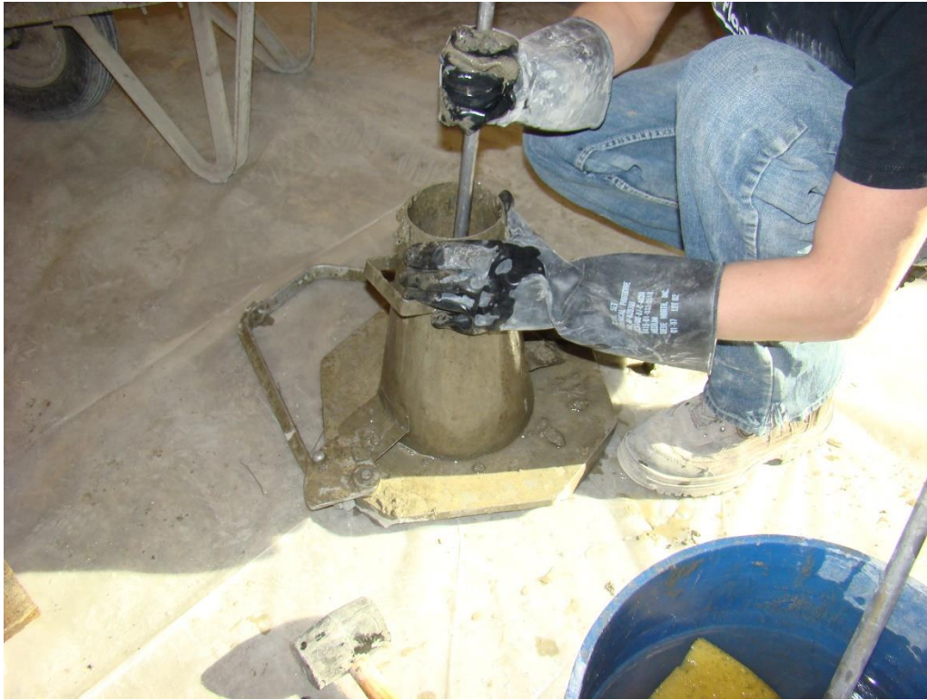
Figure 8-9: Rodding during a concrete slump test
