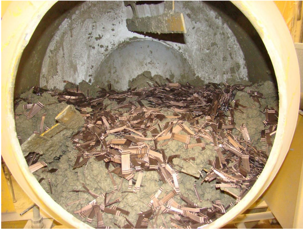
Figure 8-8: Distribution of fibers on the surface of the resting concrete, prior to the final five minutes of mixing
