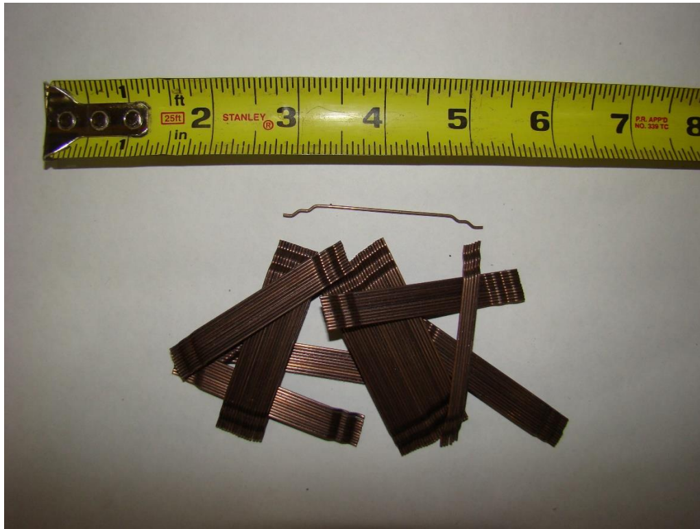
Figure 8-5: Dramix 5D fibers, manufactured by Bekaert
