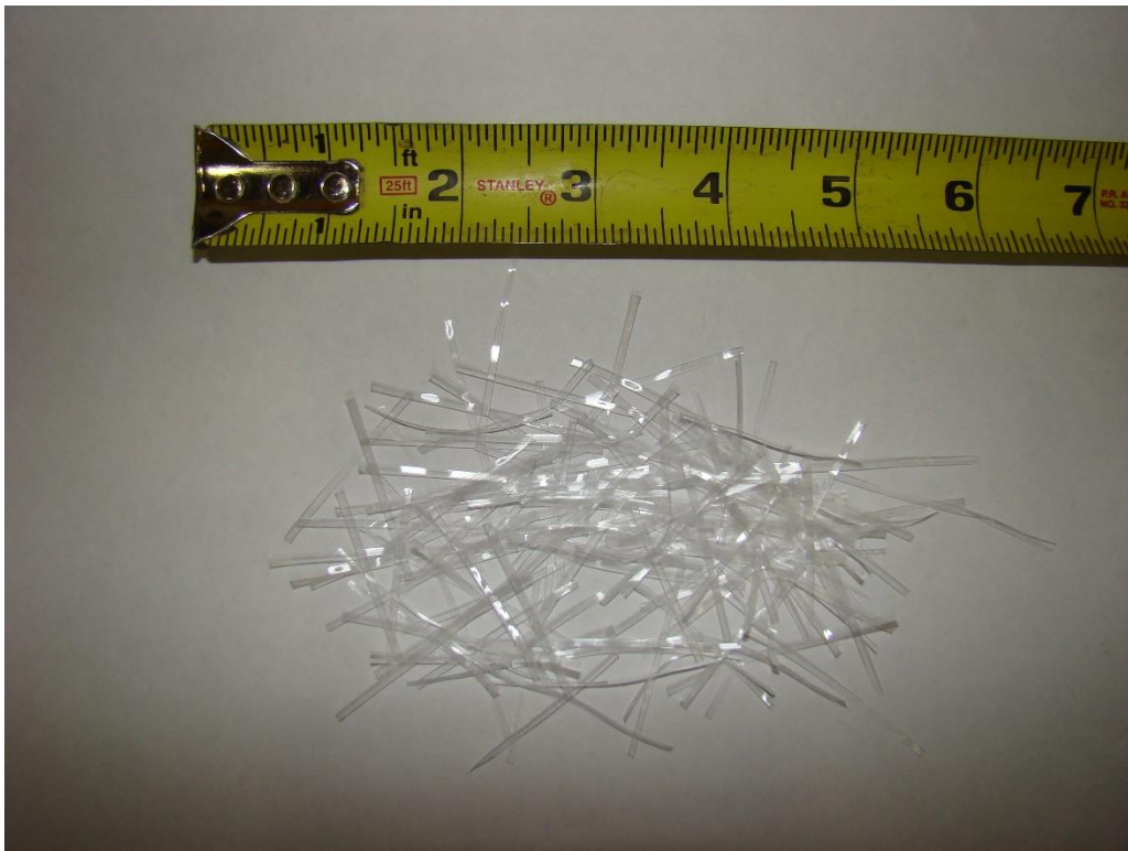
Figure 8-2: Fibermesh 650 fibers, manufactured by Propex
