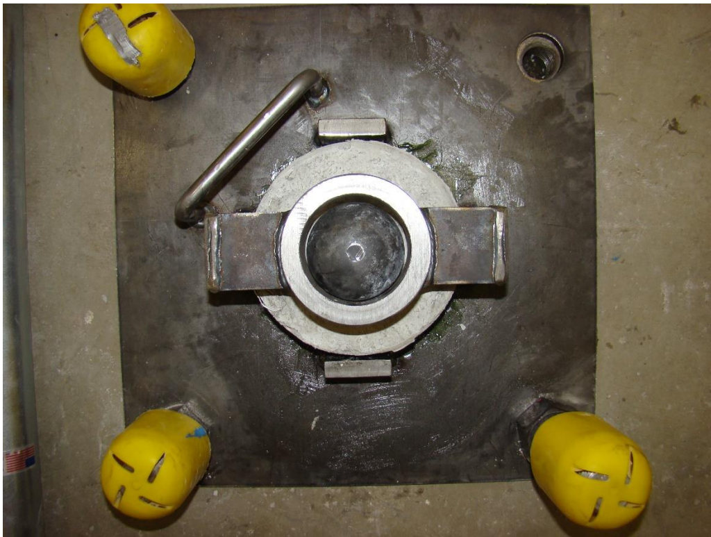
Figure 8-24: Top view of the impact strength testing setup
