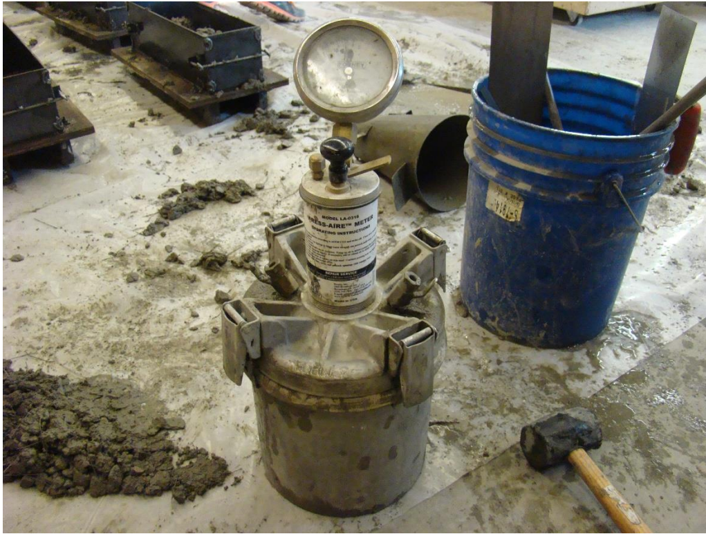
Figure 8-16: Air meter used to determine the concrete's air content, according to ASTM C231
