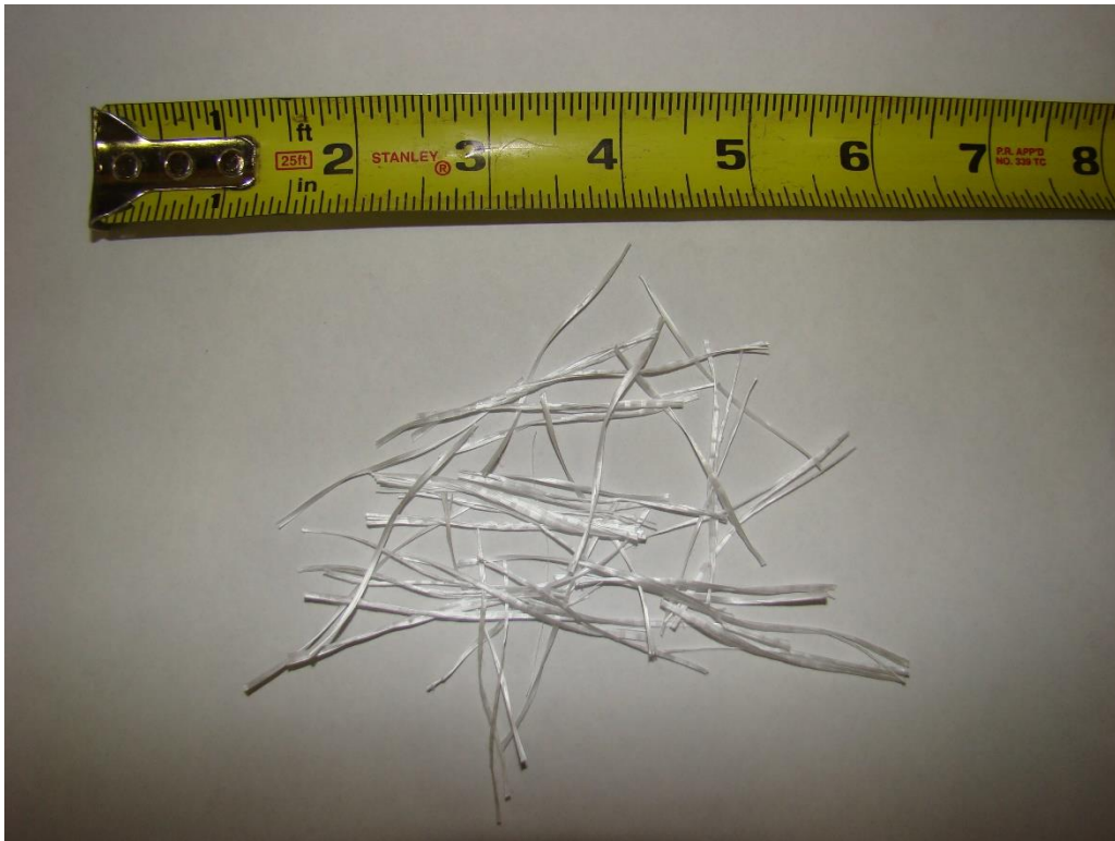
Figure 8-3: TUF-STRAND SF fibers, manufactured by The Euclid Chemical Company
