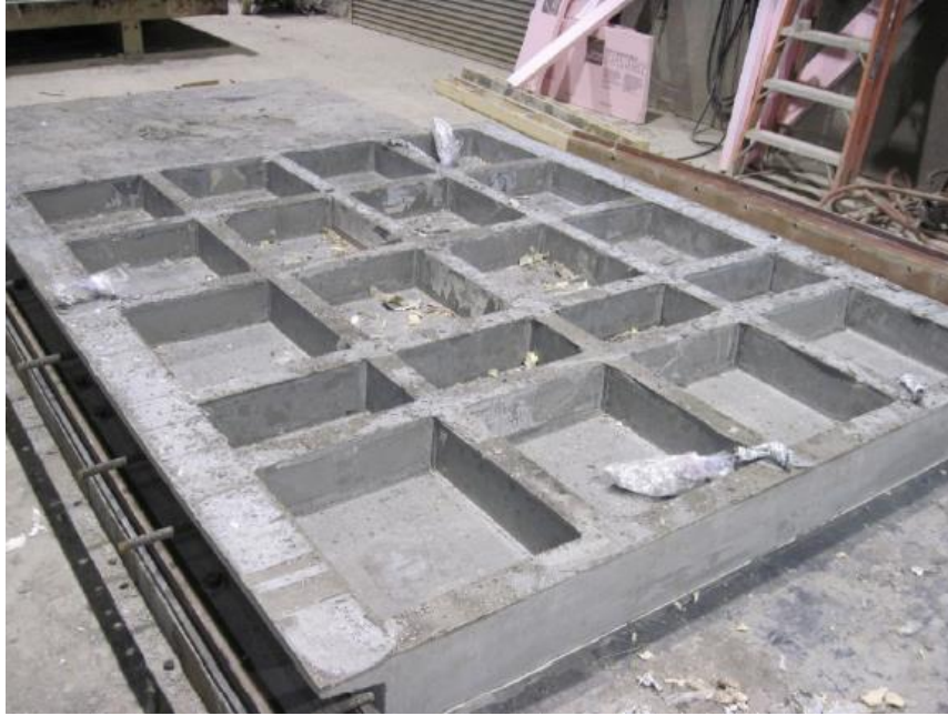
UHPC Waffle Bridge Deck Panels (Heimann 2013)
