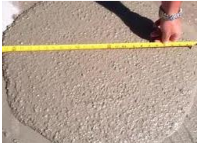
Figure 2-12: Flowability of self-consolidating concrete (SCC) (EAC, 2014)
