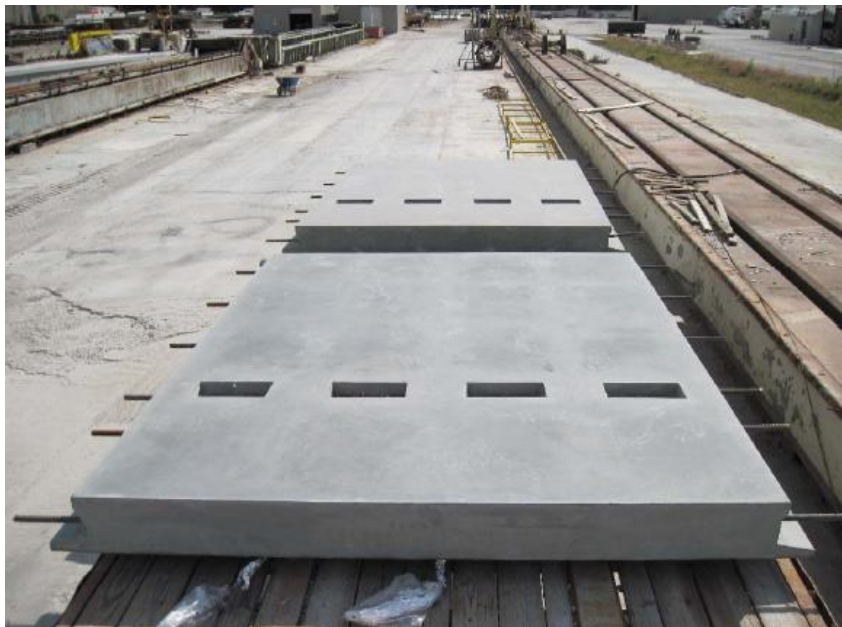
UHPC Waffle Bridge Deck Panels (Heimann, 2013)
