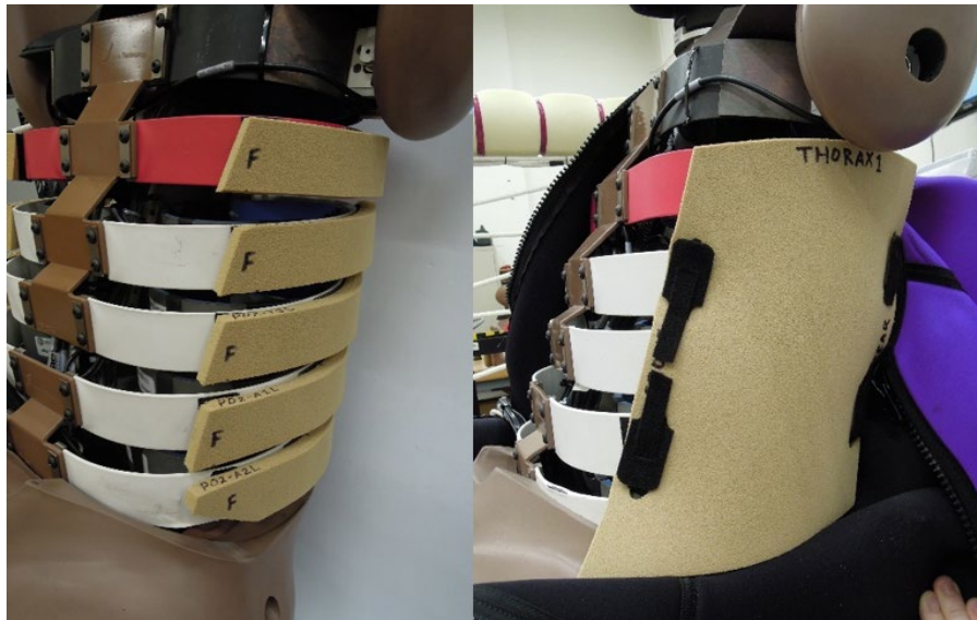
Figure 1. Split thorax pad used in the July 2022 R&R study (left). One-piece thorax pad used in the present study (right).
