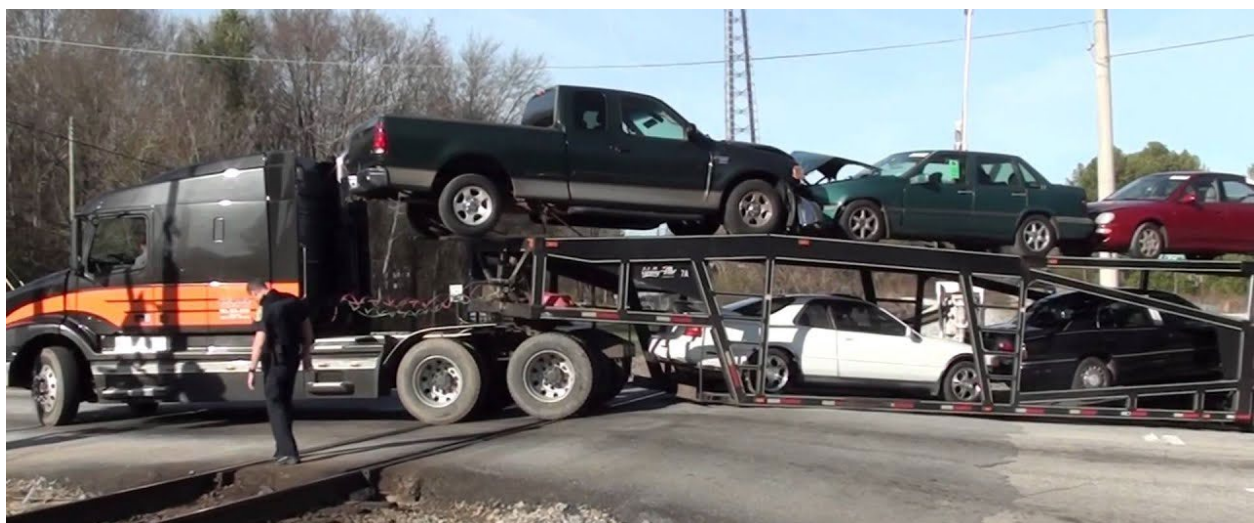
Figure 3: A automobile transport trailer stuck on a humped high-profile grade crossing
