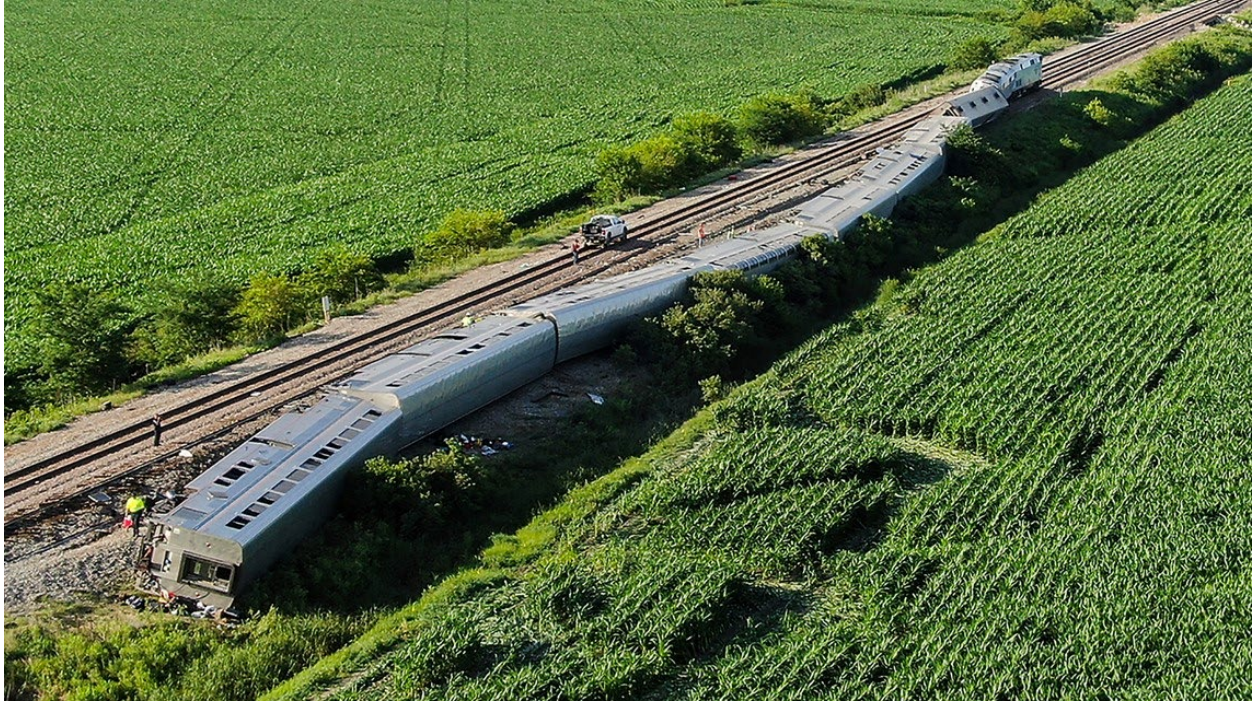
Figure 5: An Amtrak train that derailed after striking a dump truck stuck in a humped crossing
