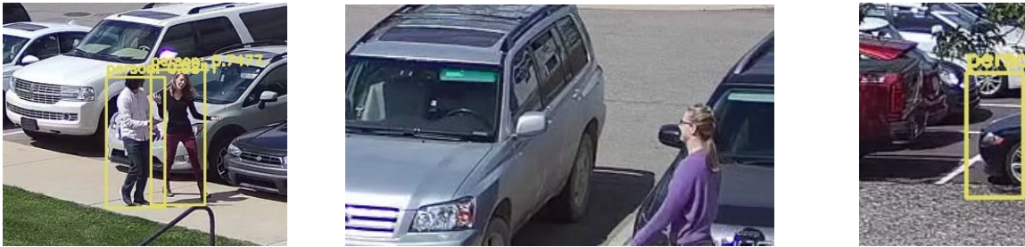
Figure 3. Results from initial testing with rooftop data collection: left – correctly detected people; middle – missed detection; right – incorrect detection
