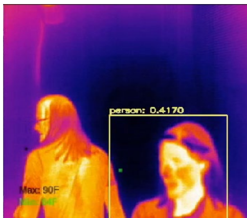
Figure 5. Thermal camera data processed using Darknet architecture
