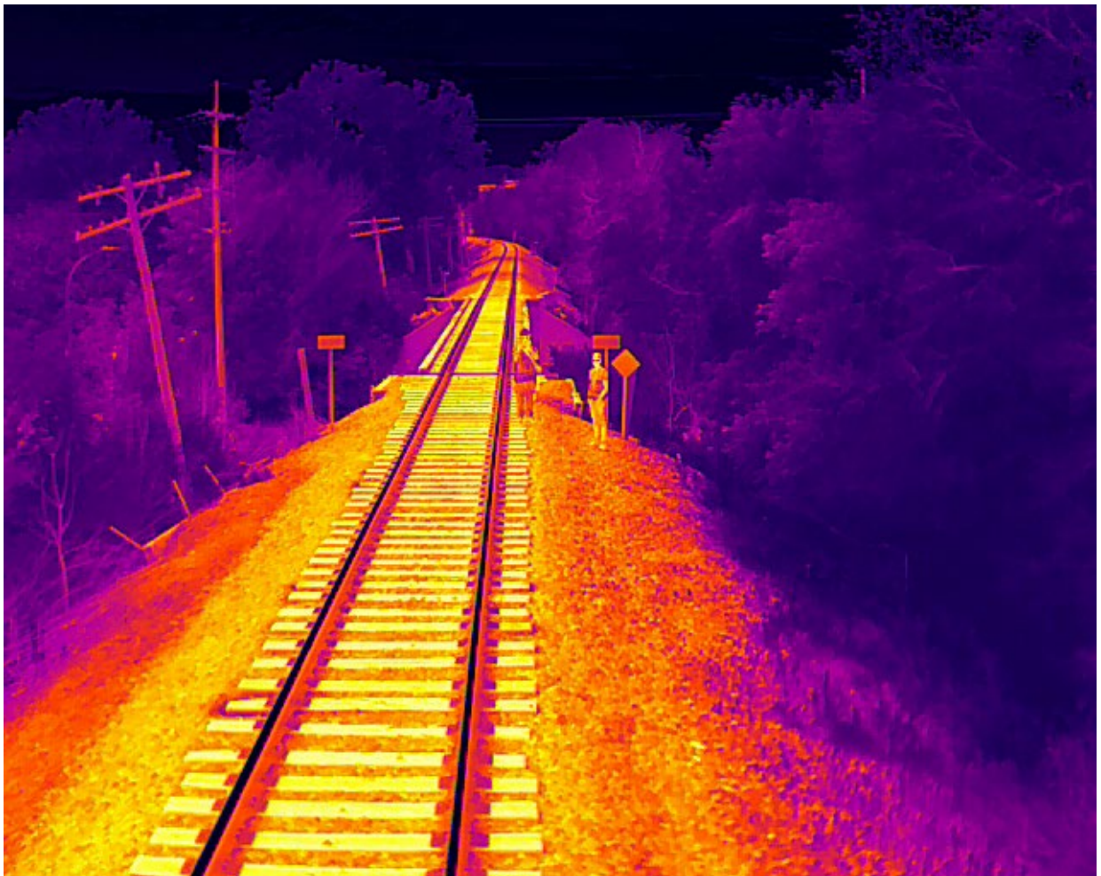
Figure 16. Simulated trespassers captured using thermal camera on UAV operating at an altitude of 25 ft.
