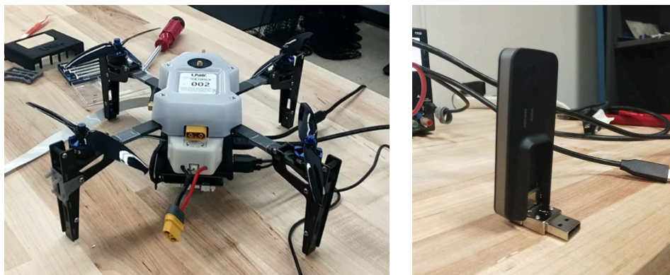
Figure 9. Left – Uvify IFO-S UAV; right – wireless cell dongle for transmission of trespasser detections
