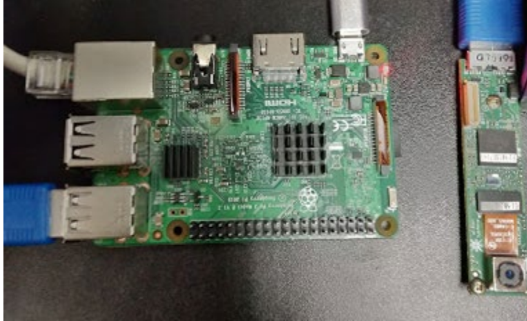
Figure 2. Raspberry Pi and camera module used for initial benchtop testing
