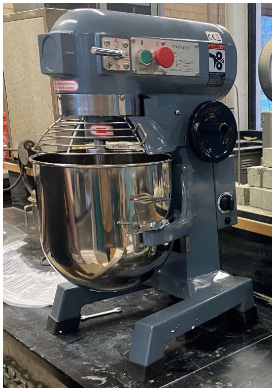
Figure 66. Photo. Benchtop mortar mixer used in the repeatability study.
