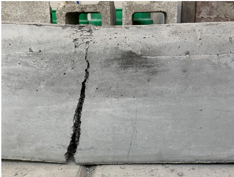
Figure 75. Photo. Flexural failure mode of beam NYTR-2.
