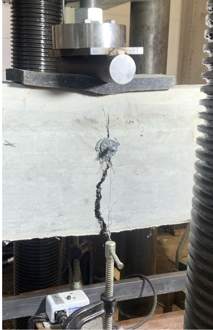
Figure 76. Photo. Flexural failure mode of beam NNTR-2.
