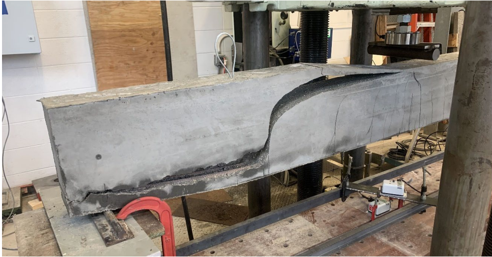
Figure 74. Photo. Shear failure mode of beam NNTR-0.
