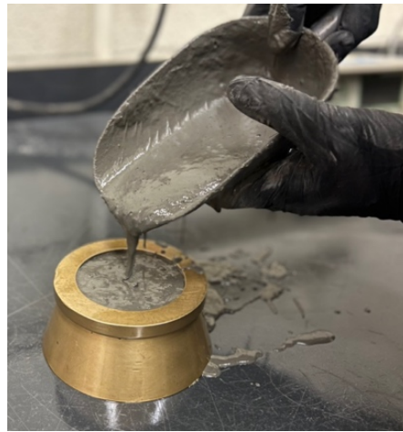
Figure 11. Photo. Mini-slump flow test used in measuring the rheological property (flow) of the fresh UHPC mixes.
