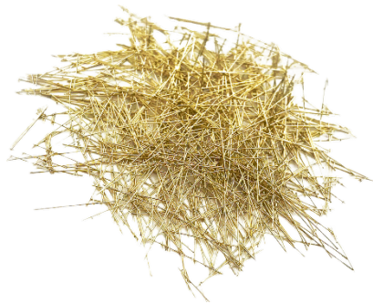
Figure 79. Photo. Striated steel fibers (0.2 mm × 13 mm) from HiPer Fibers used in the development of UHPC mix designs.
