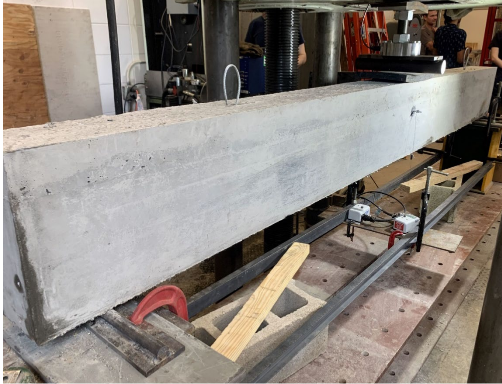
Figure 72. Photo. Beam test setup.
