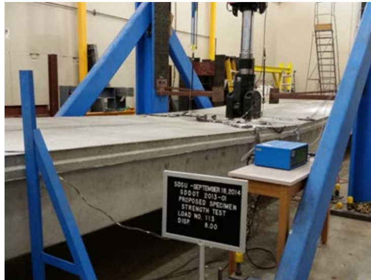
Figure 8-24: “Proposed” Specimen at Failure
