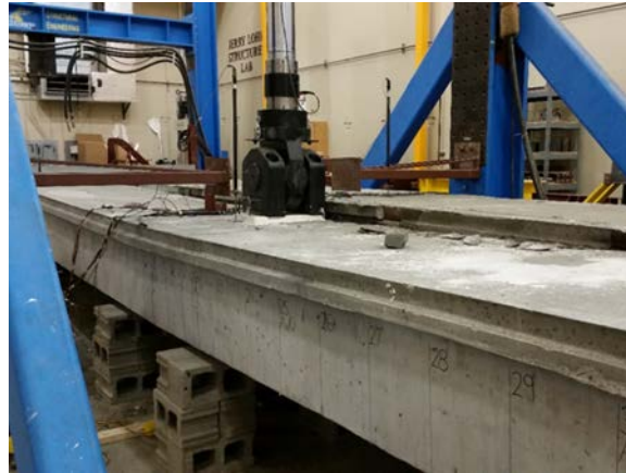
Figure 8-11: “Conventional” Specimen at Failure
