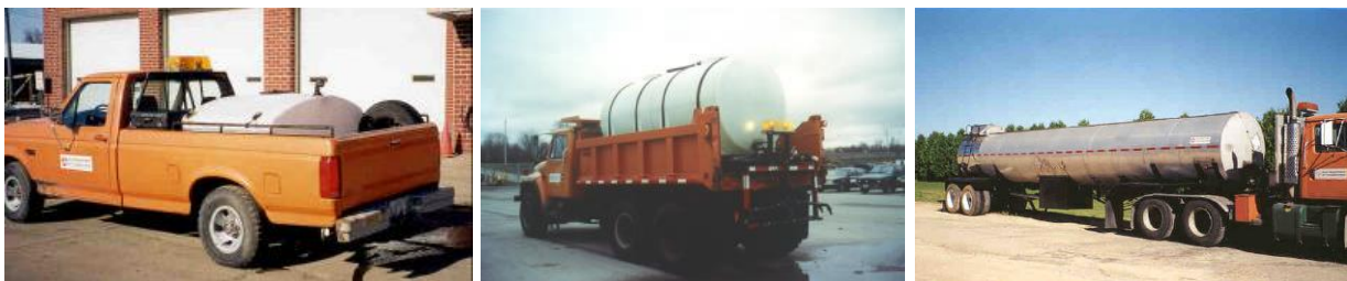
Figure 6.3 Brine spreading trucks: 250 gallons (left), 1,800 gallons (middle) and 5,000 gallons (right) (Iowa DOT)
