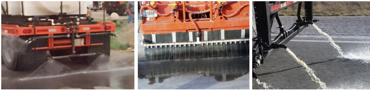
Figure 6.4 Brine spreading nozzles: fan style (left), streamer nozzle (middle) and concentrated method (right) (Iowa DOT)
