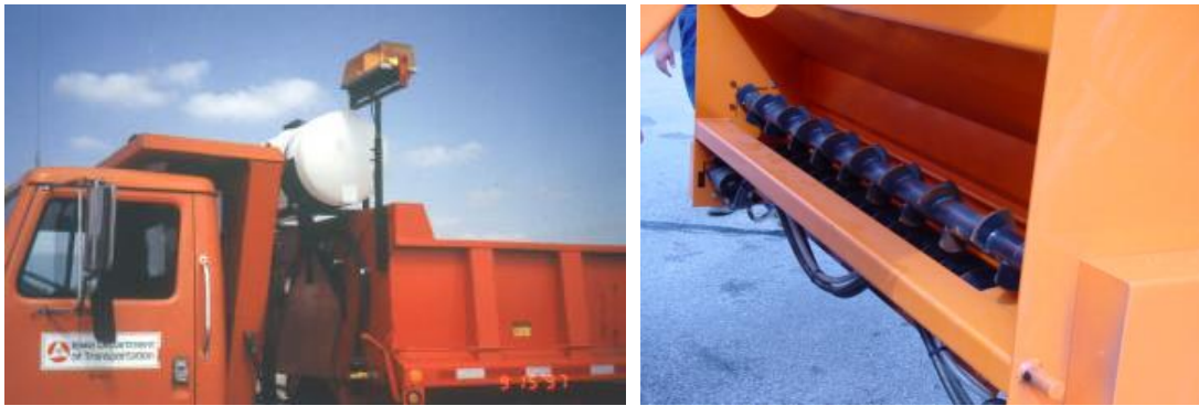
Figure 6.2 A typical truck with a brine pre-wetting unit (left) and a truck with an auger used to break up any salt clumps that may form (right) (Iowa DOT).
