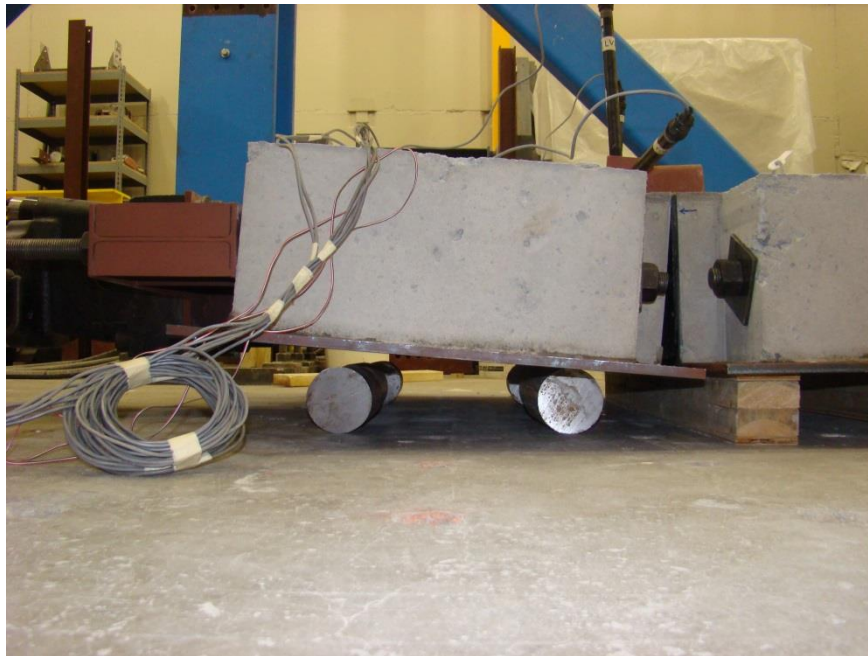
Figure 6-16: Slab Rotation During Testing of Specimen VT-4-1
