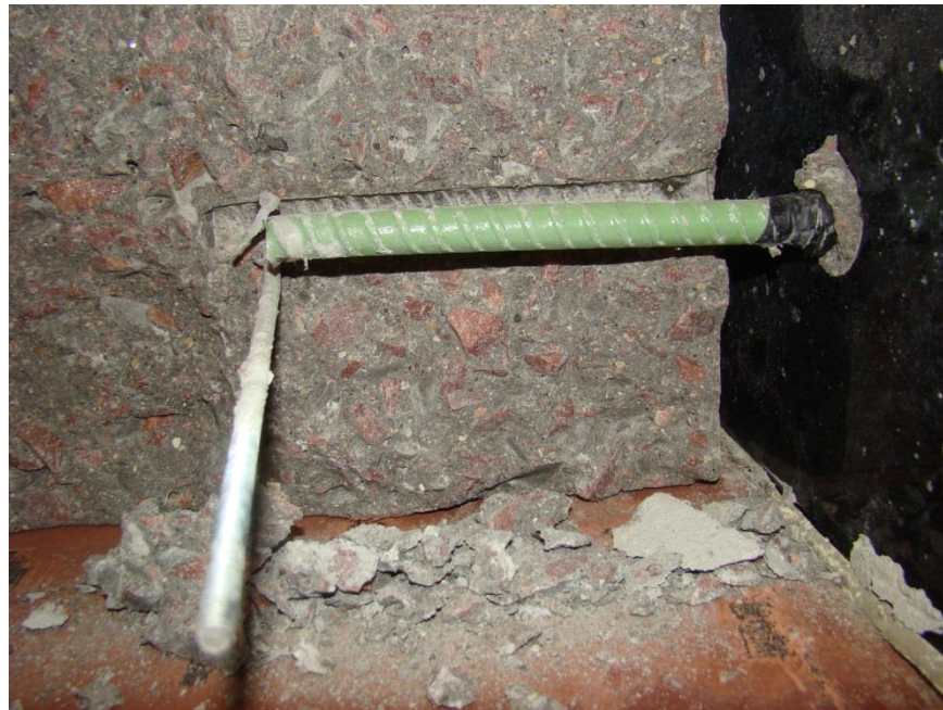
Figure 7-16: Specimen LT-7-2 Failure Plane
