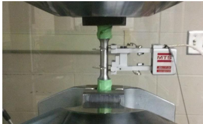
Figure 6-1: Tensile Test of a Dog-Boned Tie Bar Sample
