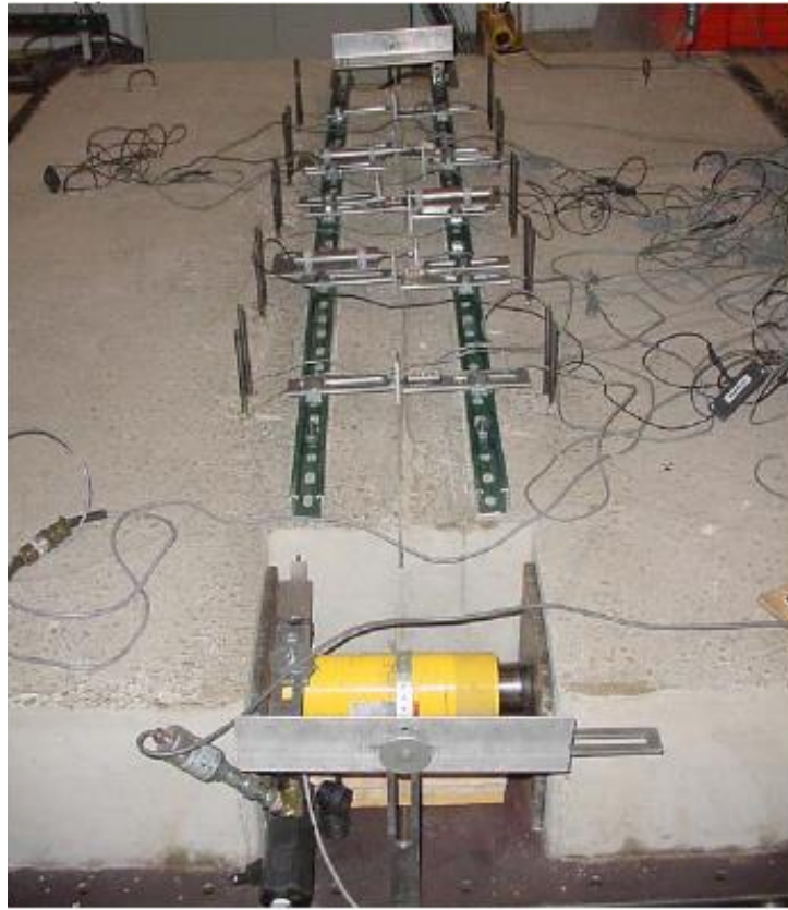
Figure 5-8: A 5-Dowel Bar Specimen (Buch, Varma, & Prabhu, 2007)
