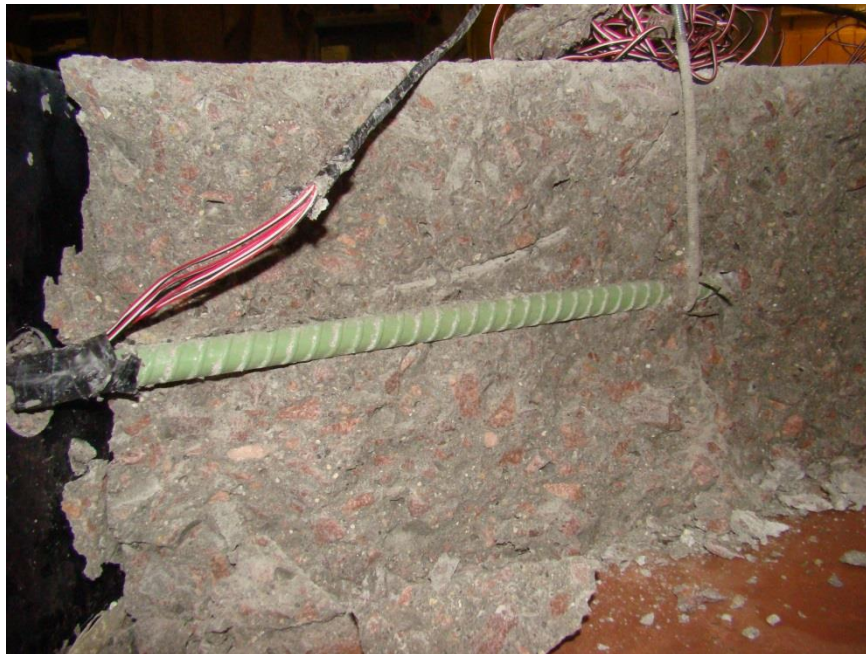
Figure 7-20: Specimen HS-16-1 Failure Plane
