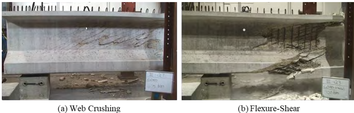
Figure 6. Photographs. Failure crack patterns for (a) web crushing and (b) flexure-shear sectional shear failures.
