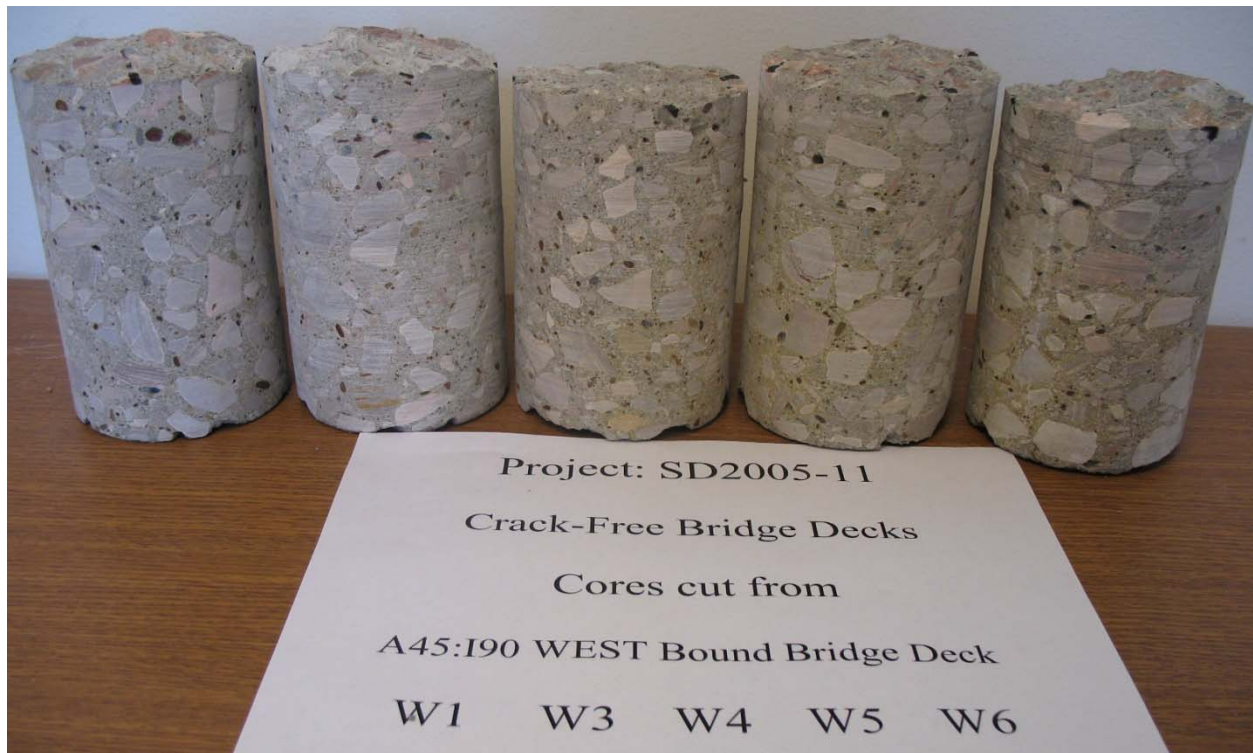
Fig. 12.7 Cores cut from Control Slab – A45 (Front)
