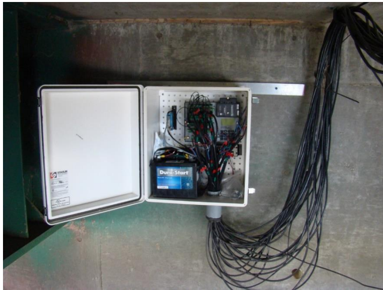
Figure 7-10: Installed Weatherproof Box for the Data Logger
