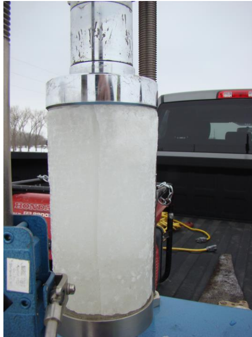
Figure 7-24: Compressive Strength Test Setup of an Ice Core Sample
