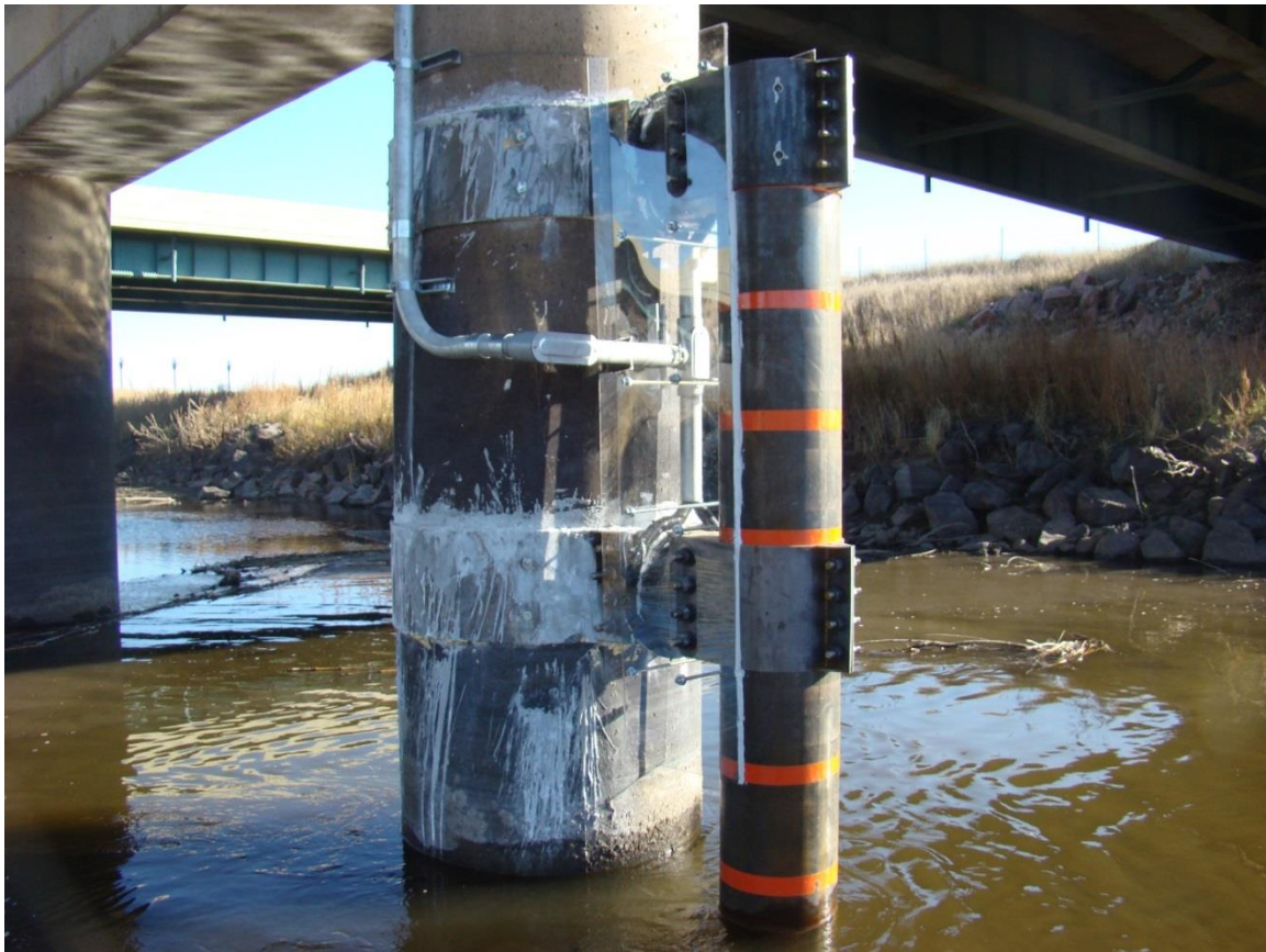
Figure 6-9: Installed Monitoring System and Protection
