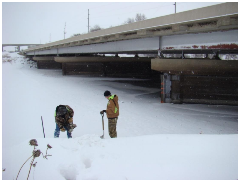
Figure 7-23: Researchers Taking Ice Core Samples at the James River Site
