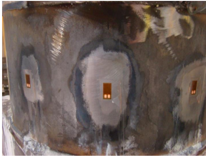
Figure 6-7: Strain Gages Applied in the Center of the HSS Load Cell
