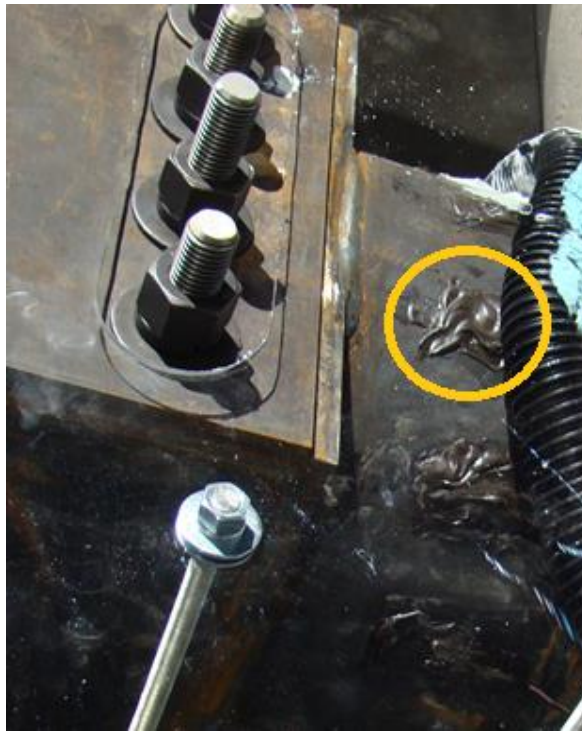
Figure 6-8: Load Cell with the Strain Gage Protection (Highlighted)
