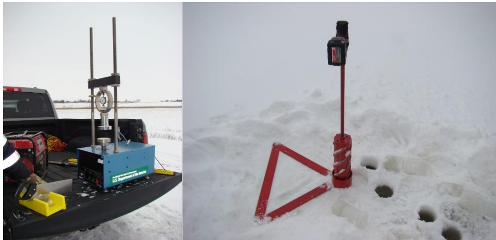
Figure 7-22: Equipment for Ice Coring and Measurement of Ice Strength
