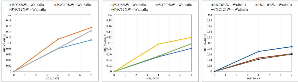
Figure 414 The Effect of Cement Content on Free Shrinkage at 8%, 10% and 12% water content.
