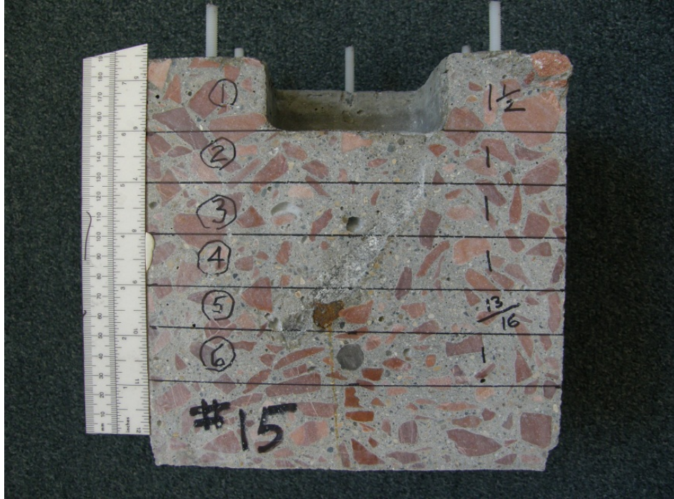
Figure 5-17: Horizontal slice scheme for concrete specimen
