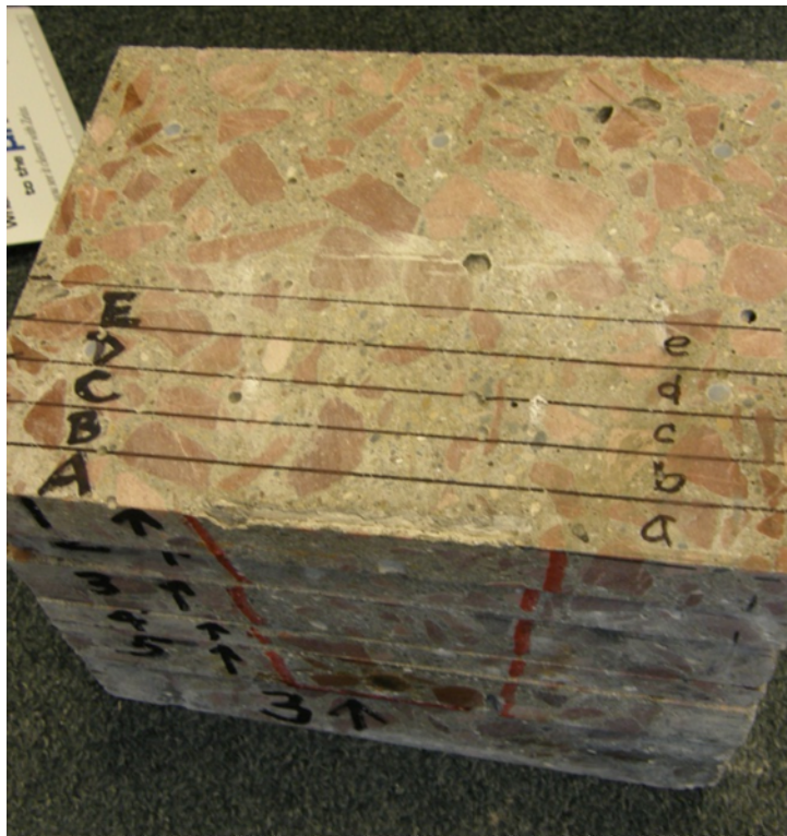
Figure 5-18: Vertical slice scheme for concrete specimen
