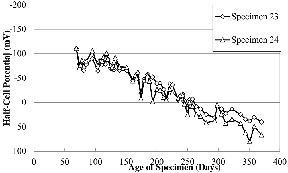
Figure 6-81: Half-cell potential measurements for uncracked, control specimens
