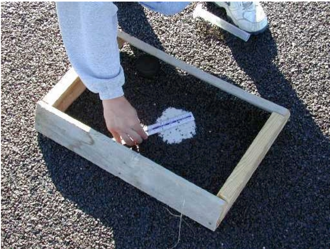
Figure A-22. Measurement of diameter for sand patch test.
