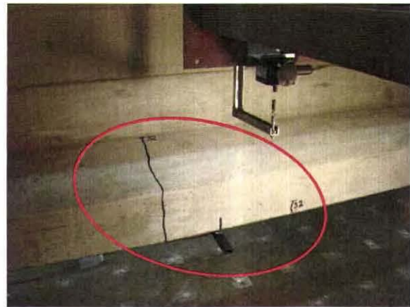
(b) First Flexural Cracks at Load = 161 Kips
