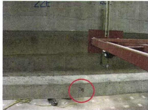
(b) First Flexural Crack at Load = 157 Kips
