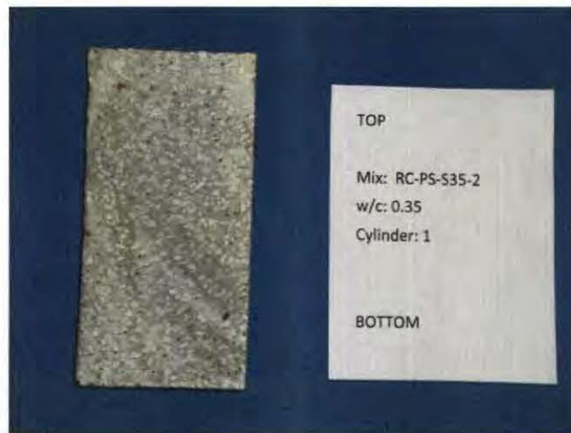
Figure 6.35: Sawn Cylinder for HVSI Evaluation
