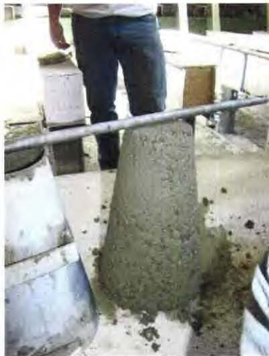
(a) Slump Test of Conventional Concrete
