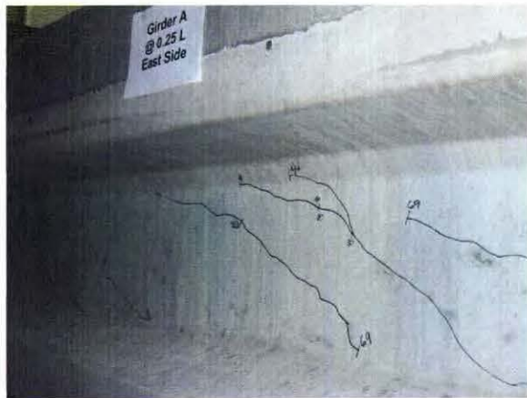
(c) Development of Diagonal Shear Cracks
