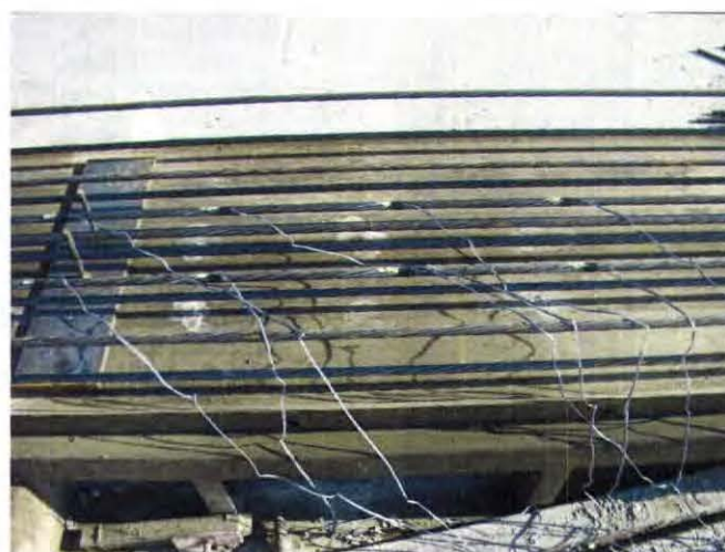
Figure 7.7: Transfer Length Strain Gages
