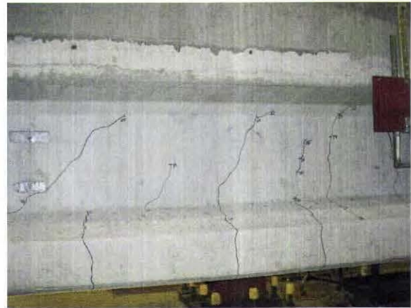
(b) Development of Flexural-Shear Cracks
