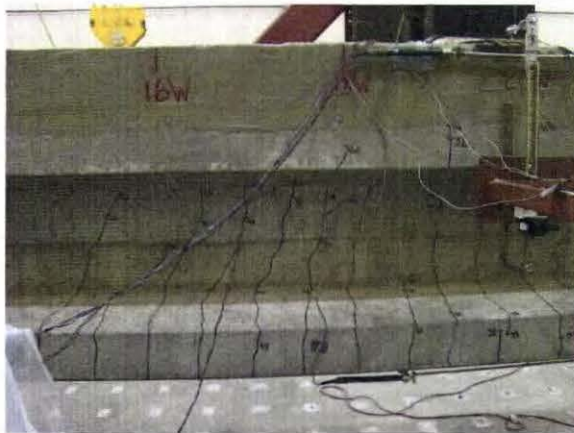
(c) Flexural and Flexural-Shear Cracks
