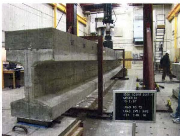
(e) Girder BL Shortly before Failure
