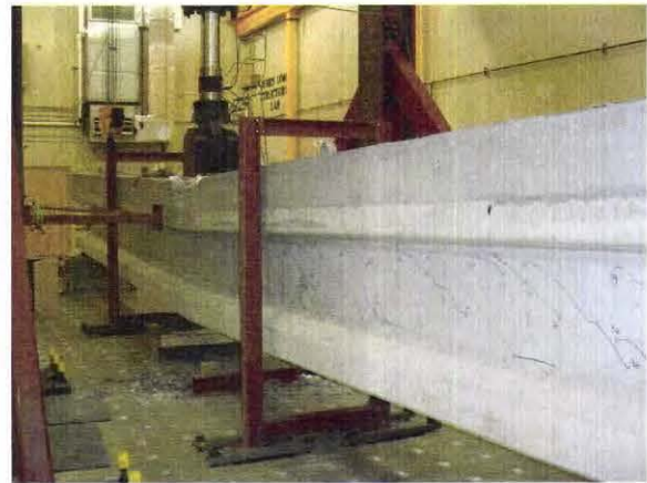
(d) Crushing of Compression Concrete at Failure
