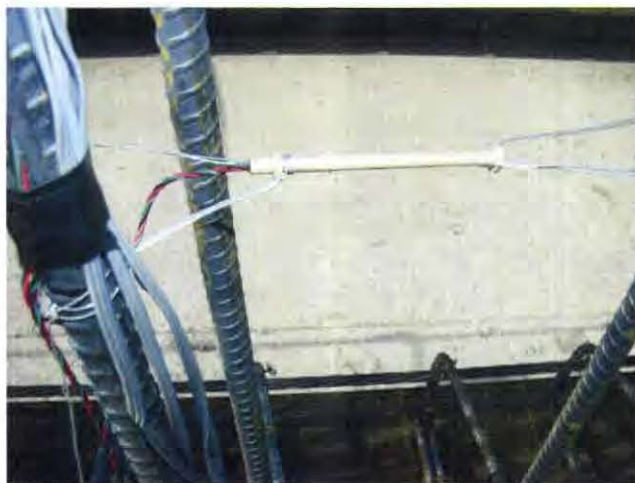
Figure 7.8: Embedded Strain Gage
