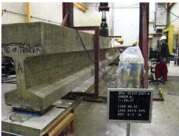
(e) Girder AL Shortly before Failure
