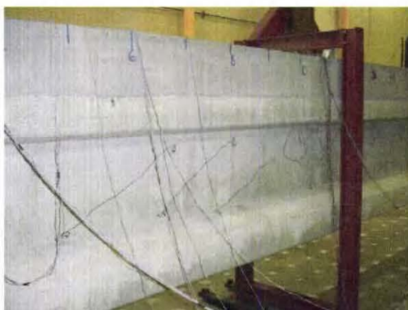
(c) Development of Diagonal Shear Cracks
