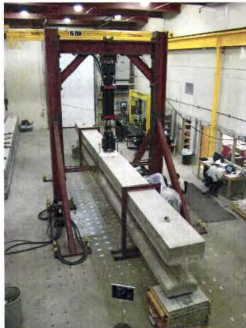
Figure 7.18: Test Set Up of a Girder Specimen
