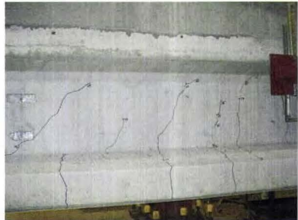
(b) Development of Flexural-Shear Cracks
