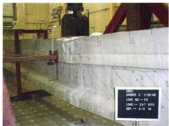
(d) Crushing of Compression Concrete at Failure
