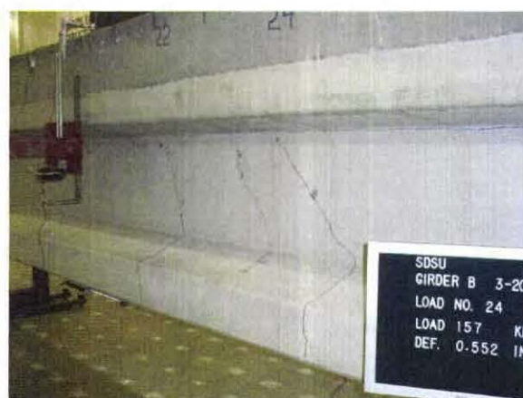
(b) Development of Flexural-Shear Cracks
