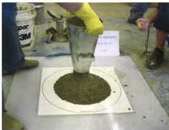
Figure 5.1: Slump Flow Test
