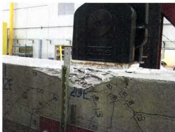
(f) Crushing of Compression Concrete at Failure
