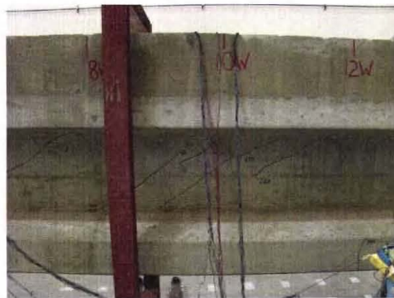
(e) Diagonal Shear Cracks at Load = 232 Kips
