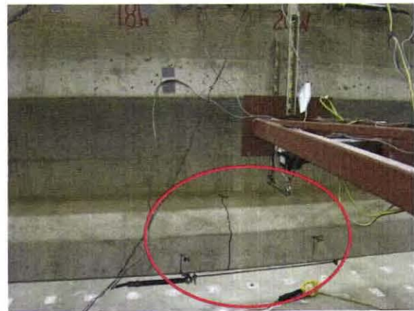
(b) First Flexural Cracks at Load = 153 Kips
