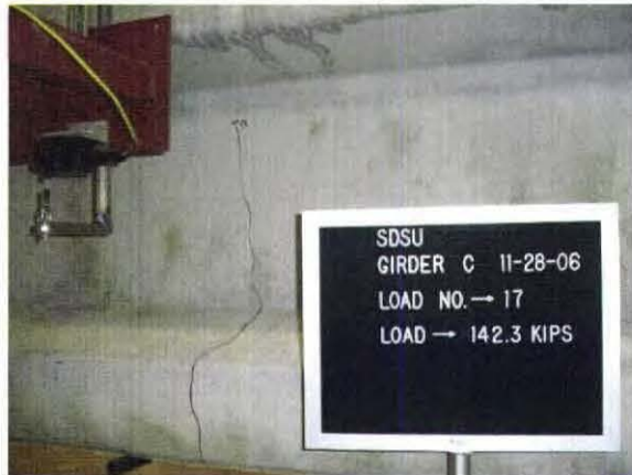
(a) First Flexural Crack at Load = 143 Kips
