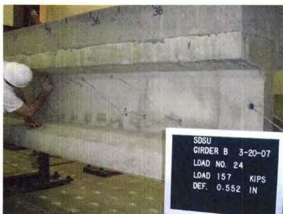
(c) Development of Diagonal Shear Cracks
