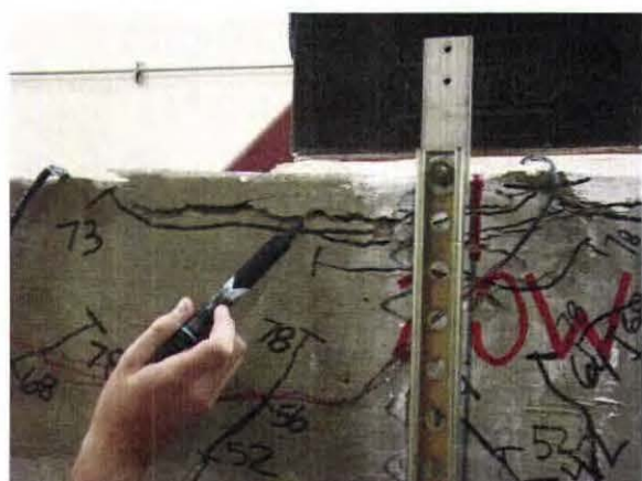
(f) Crushing of Compression Concrete at Failure
