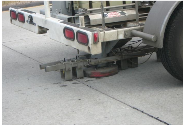
Figure 7.23: FWD Test at a Transverse Joint
