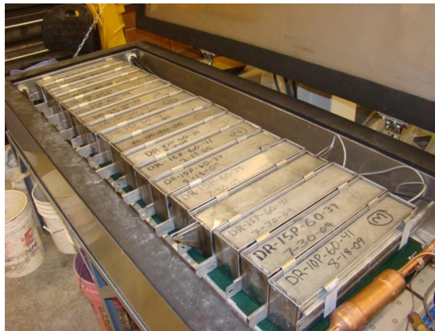
Figure 6.19: Beam Specimens in the Freeze-Thaw Cabinet
