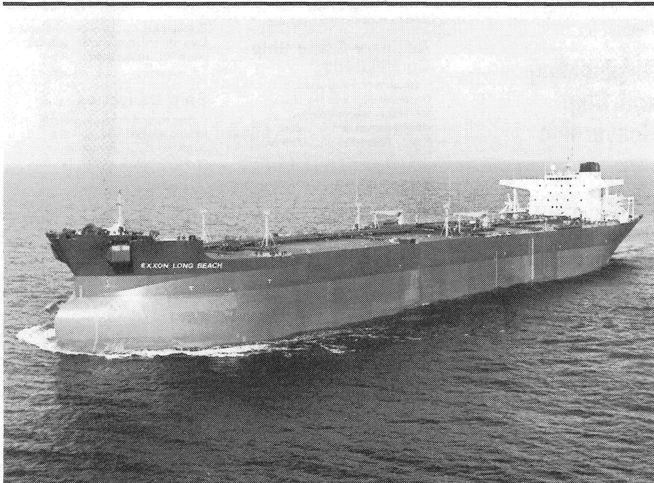
The EXXON LONG BEACH, second of three 209, 200-deadweight-ton crude oil tankers built for Exxon Shipping Co., by National Steel and Shipbuilding Co., during sea trials. The vessel was delivered in March 1987.
