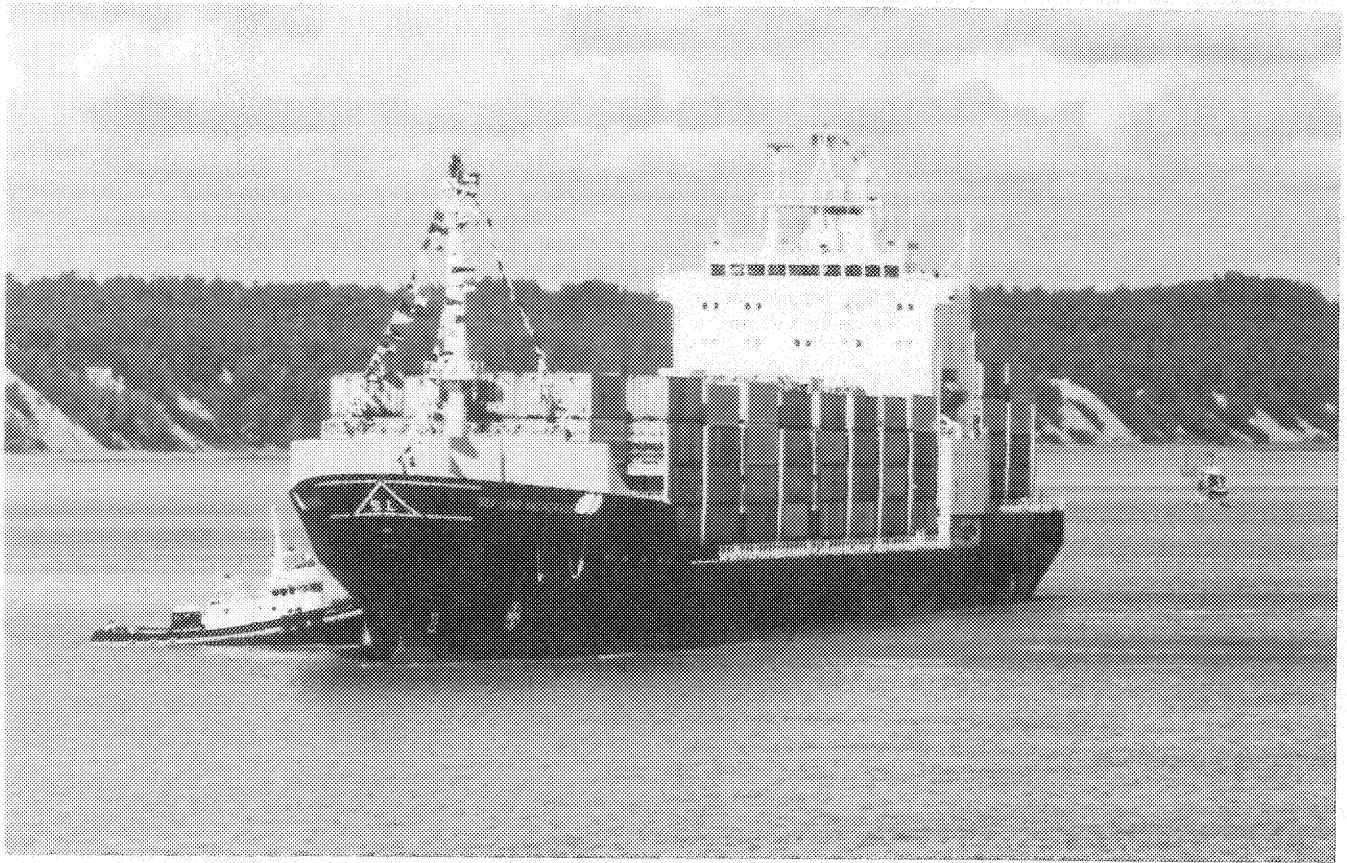
The 21,000-deadweight-ton containership, SEA-LAND ANCHORAGE, was built by Bay Shipbuilding Corp. and delivered in fiscal year 1987.
