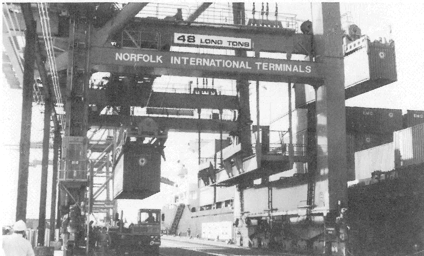
One of three high-speed, dual-hoist container cranes in operation at Norfolk International Terminals. These cranes were designed to allow as many as 50 container movements per hour, or almost double the rate of conventional cranes.
