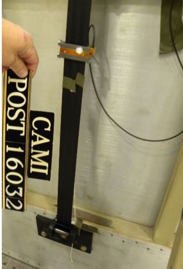
Figure 13: Shoulder Belt Showing String in Foam and Lower Webbing Transducer
