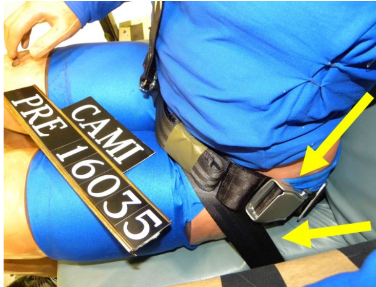
Figure 6: Configuration 1 Belt Routing, Highlighting Conventional and Body-Centered Lap Belts (Arrows)
