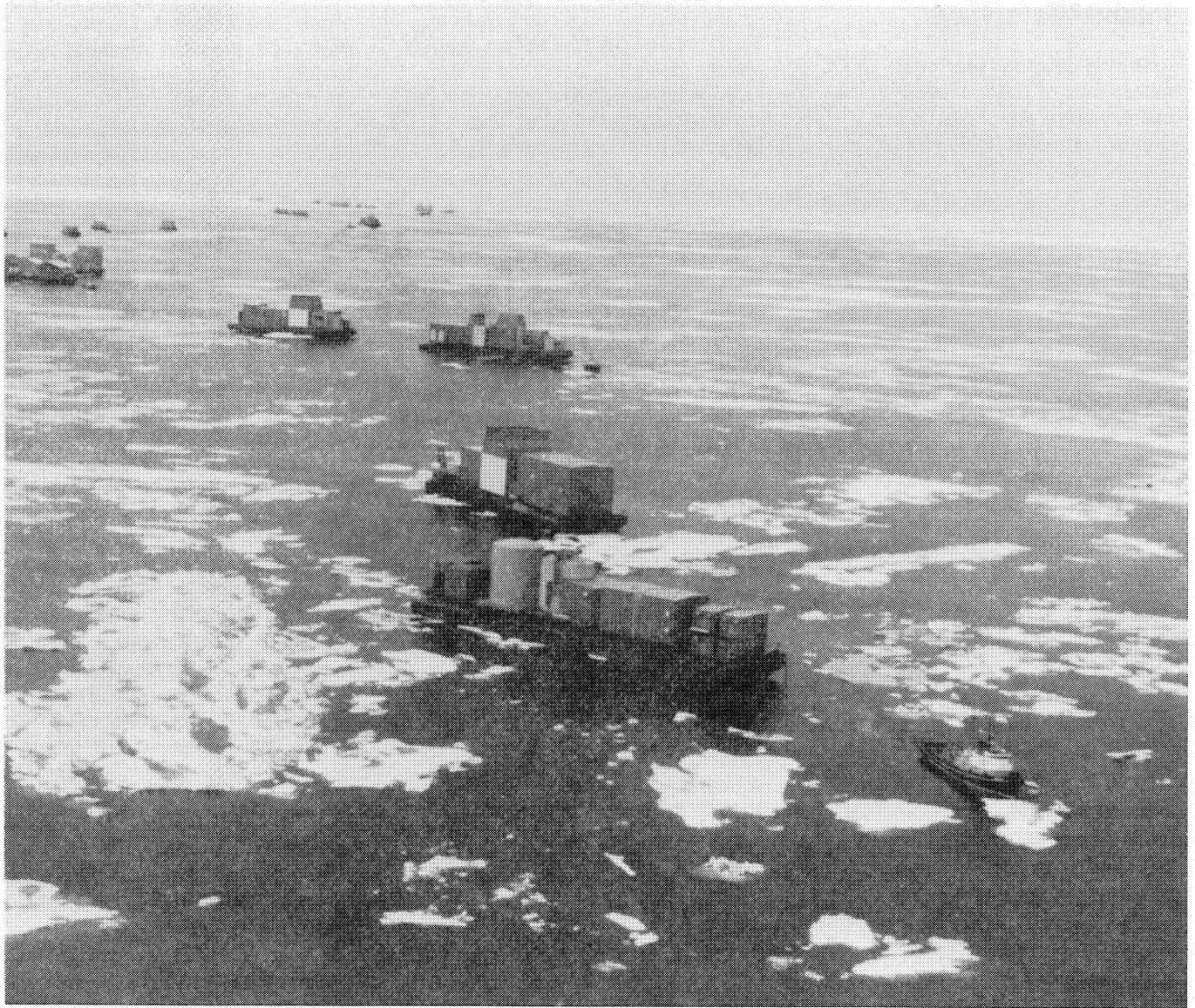
Crowley Maritime Corp.'s 1983 summer sea-lift of oil industry cargo for Alaska included 26 loaded barges, 14 tugboats, an icebreaker barge, and a salvage vessel. The fleet, carrying 96,611 tons of cargo, is shown arriving at the Beaufort Sea.
