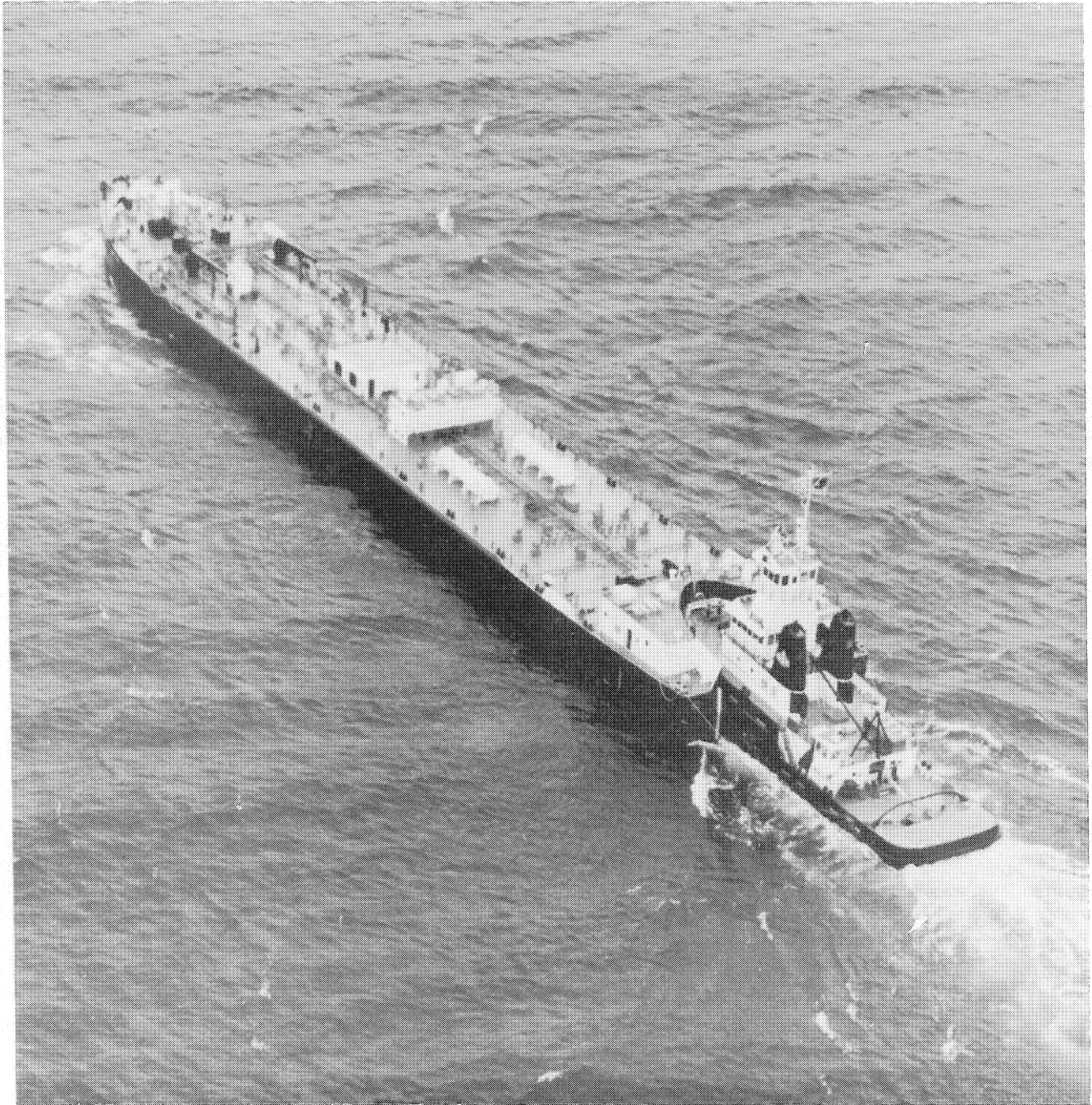
The 9,500-deadweight-ton tug/barge AMOCO GREAT LAKES/AMOCO MICHIGAN was built in 1982 by Bay Shipbuilding Corp. for Amoco Oil Co. for service on the Great Lakes.
