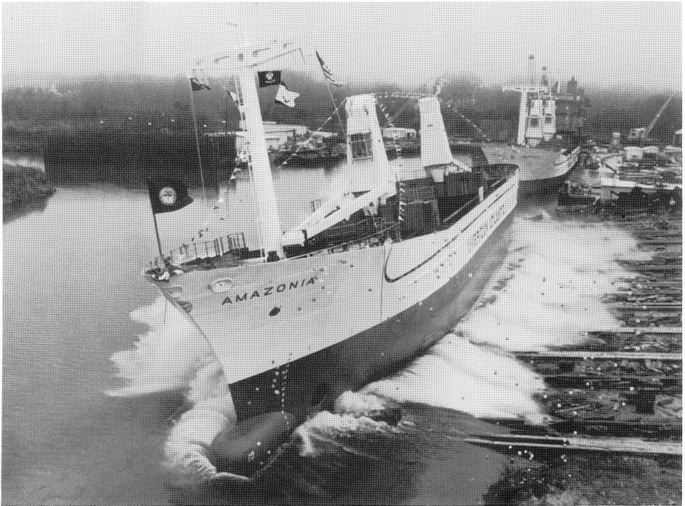
M/V AMAZONIA, second in series of 2,000-dwt. multipurpose cargo ships built for operation by American Atlantic Shipping, Inc., in Caribbean and South Atlantic trades, is launched at Equitable Shipyards, Madisonville, La., Jan. 20, 1979.
