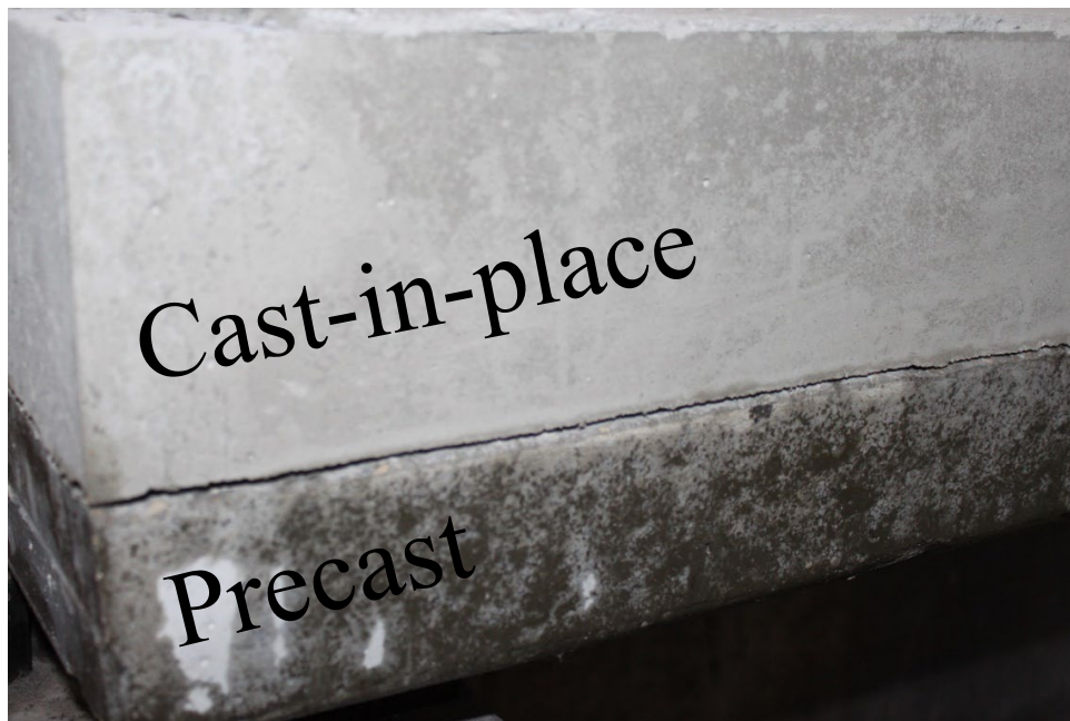
Figure 3.5 Unmodified test specimen delamination at 1.2 inches of displacement (location: northwest)
