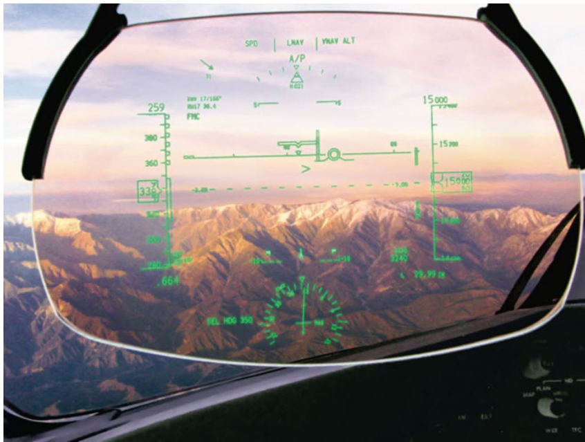
Figure 19. B787 Head-Up Display (HUD)
