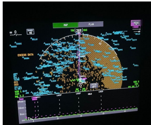
Figure 55. B787 Navigation Display (with all drop-down menu items selected) (source: personal photo)
