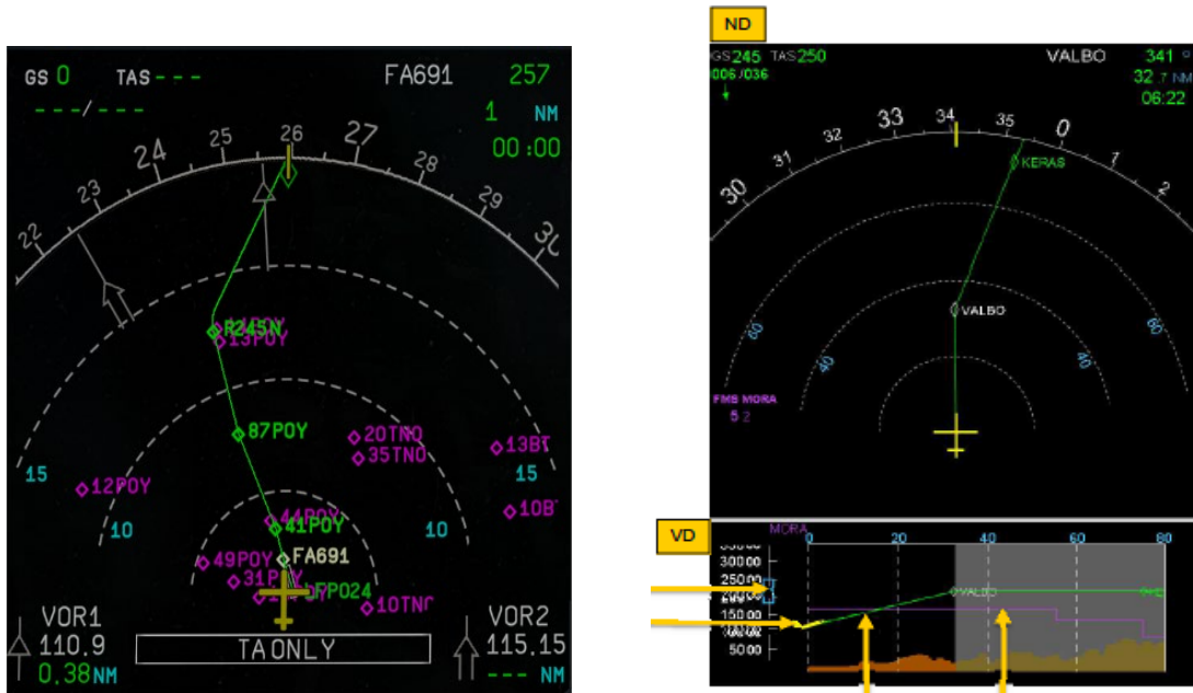
Figure 36: A320 ND in ARC Mode (left) (source: Airbus, 1998) vs. A350 ND & VD in ARC Mode (right) (source: Airbus, 2011)
