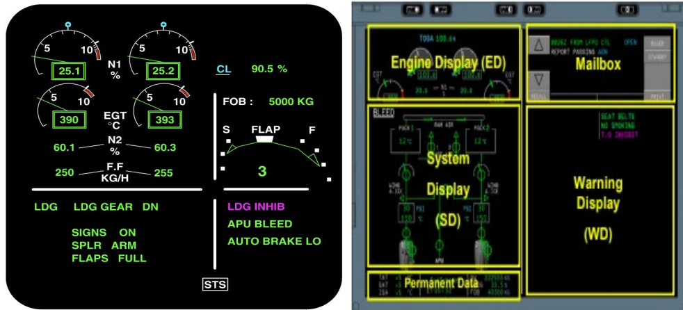
Figure 41: A320 Upper ECAM (left) (source: Airbus, 1998) vs. A350 Upper ECAM (right) (source: Airbus, 2011)
