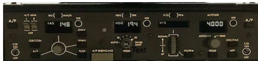
Figure 17. B787 Mode Control Panel (MCP) (source: personal photo)
