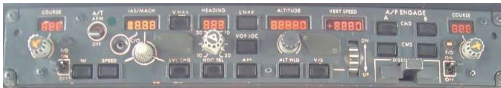
Figure 16. B737-500 Mode Control Panel (MCP) (source: http://www.b737.org.uk/images/glare-500.jpg )
