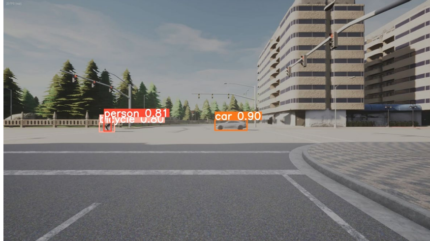
Figure 2.2: Yolo-v8 bicyclist and vehicle detection. There is a bicycle followed by a vehicle. The bicyclist is also identified as a person. Both the bicyclist and vehicle are moving along the cross street in a T-shaped intersection.
