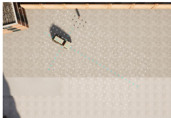
Figure 4.8: Occupancy grid 2-D array with 30° yaw angle [36].
