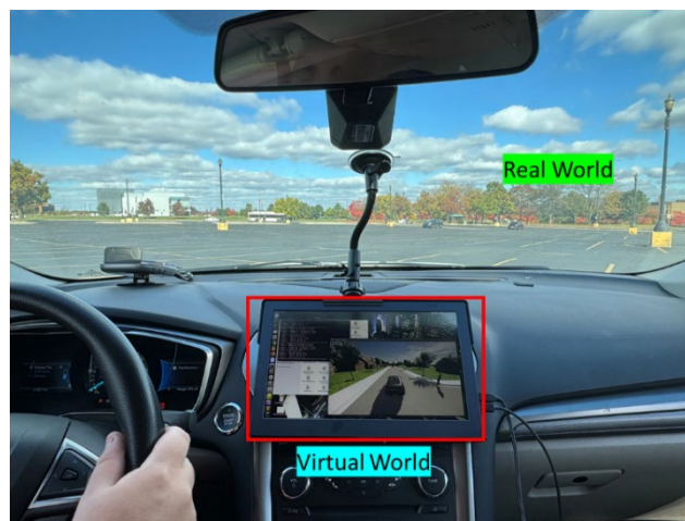
Figure 5.11: VVE real-virtual motion synchronization [45].
