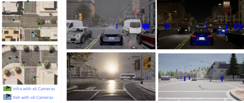
Figure 2.5: Dataset generation setup and sample images. Left: Bird’s-eye views of intersections showing infrastructure (green) and vehicle (blue) agents, each equipped with six cameras. Right: Four sample images showcasing diverse scenarios: rainy conditions (top-left), nighttime scene (top-right), sun-glare effect (bottom-left), and sunny daytime traffic (bottom-right). Blue bounding boxes indicate pedestrians. These images demonstrate challenging scenarios including occlusions, varying lighting conditions, and complex urban environments, crucial for training robust collaborative perception models.
