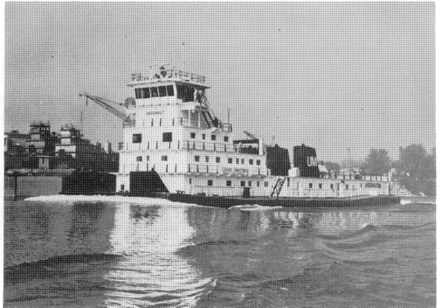
The 10,500 h.p. towboat ARGONAUT, shown as she departed from the Dravo shipyard where she was built.
