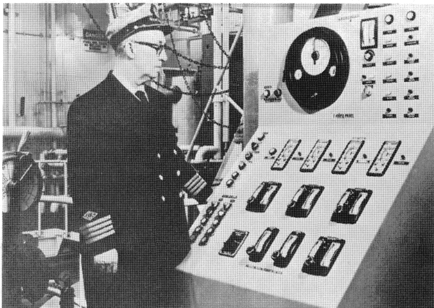
Chief engineer inspecting combustion controls of a Great Lakes vessel.
