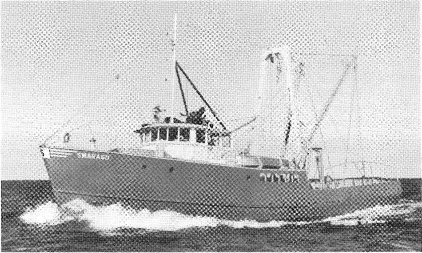
A steel scalloper, built under the direction of the Maritime Administration as part of the Department of the Interior's fishing vessel program.
