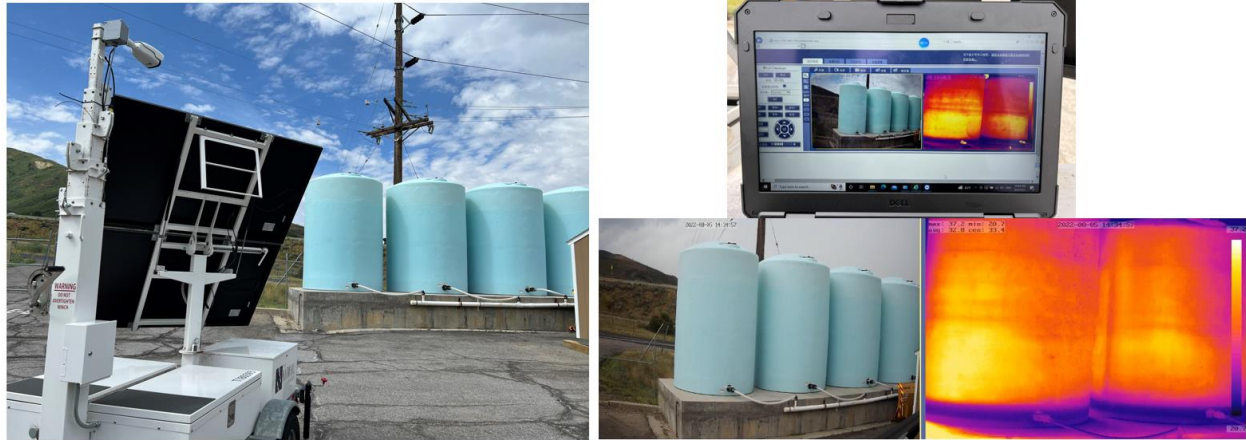
Figure 4-4 Dual-spectrum camera mounted on the portable trailer (left) and typical data collected at the UDOT Parley Springs Maintenance Shed.
