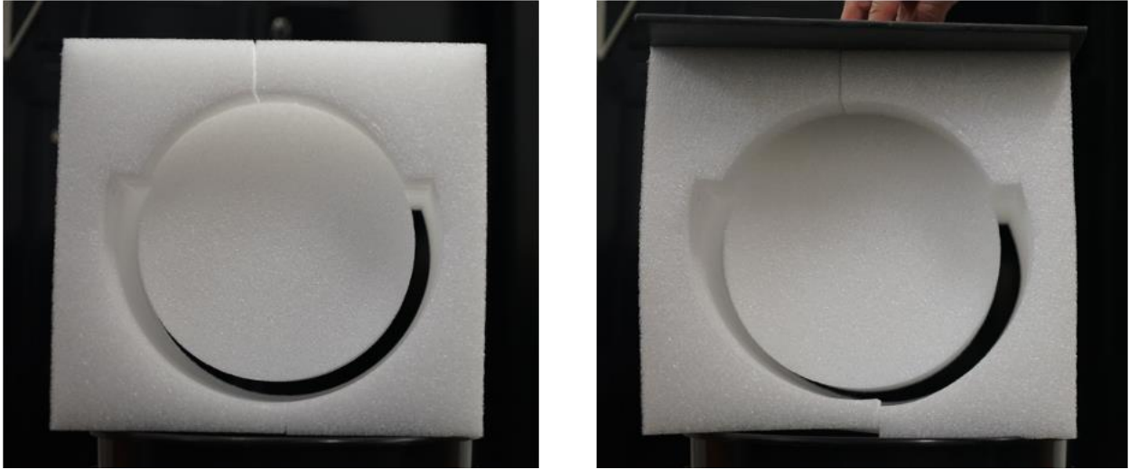
Figure 3-8 The image captured using a Sony optical camera of (a) an undeformed foam cube and (b) a deformed foam cube.
