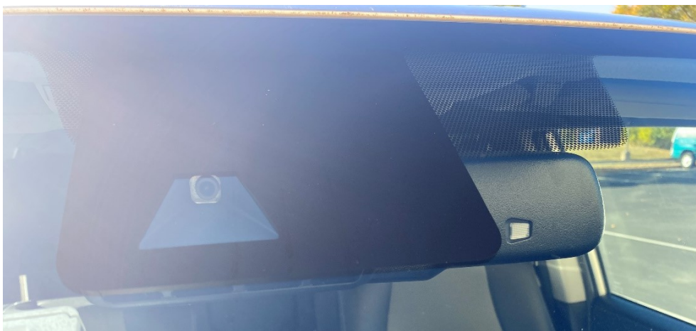
Figure 27. Toyota forward facing camera.
