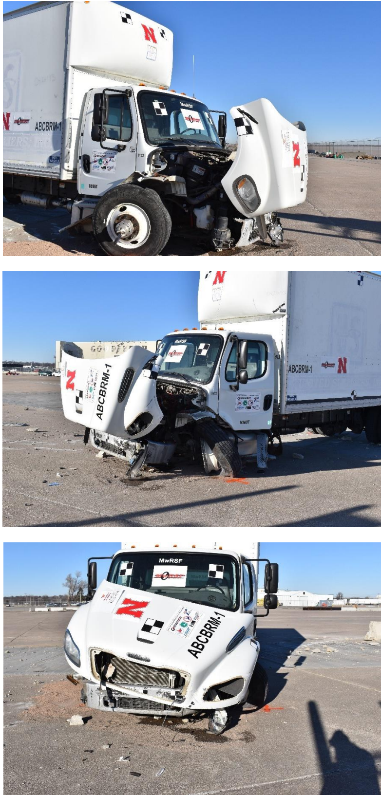
Figure 97. Vehicle Damage – Front End, Test No. ABCBRM-1
