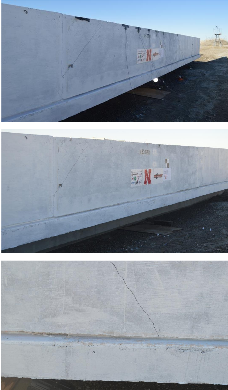
Figure 92. System Damage, Backside of Bridge Rail, Test No. ABCBRM-1
