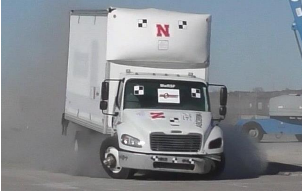
Figure 95. Vehicle Damage after Primary Impact
