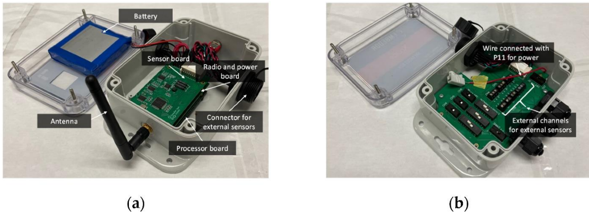
Figure 5.2. Xnode wireless smart sensor platform: (a) Xnode sensor node and (b) breakout box
