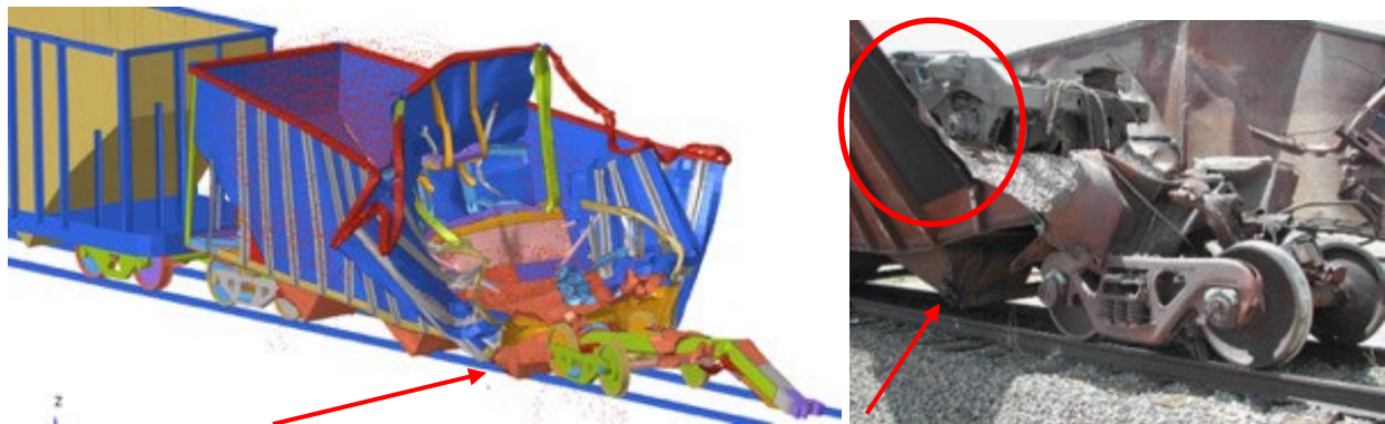
Figure 32. Post-Impact Crush Comparisons, Close-Up
