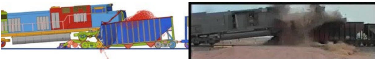
Figure 27. Sequential Images between Simulation and TTC Crash Test at 1,600 ms
