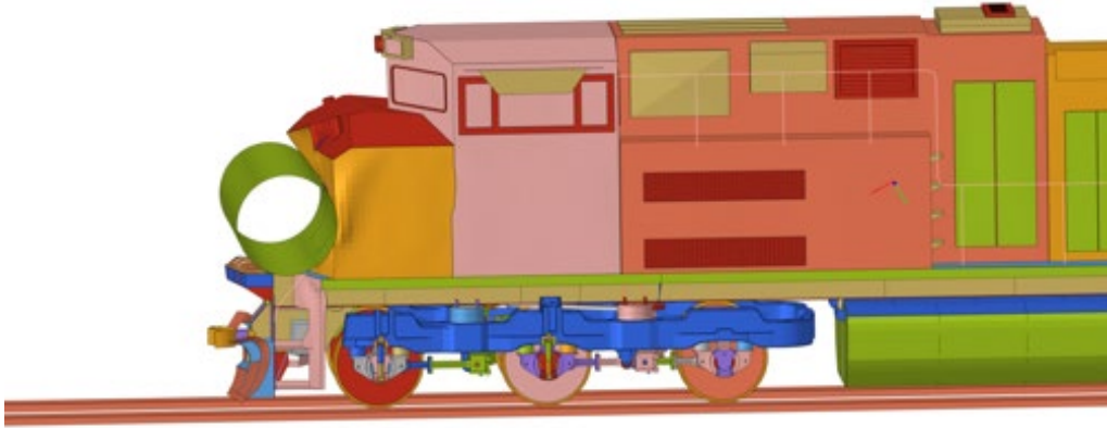
Figure 120. S-580: Cylindrical Shape Simulation Sequential Images for non-modern Locomotive Regulations at 200 ms
