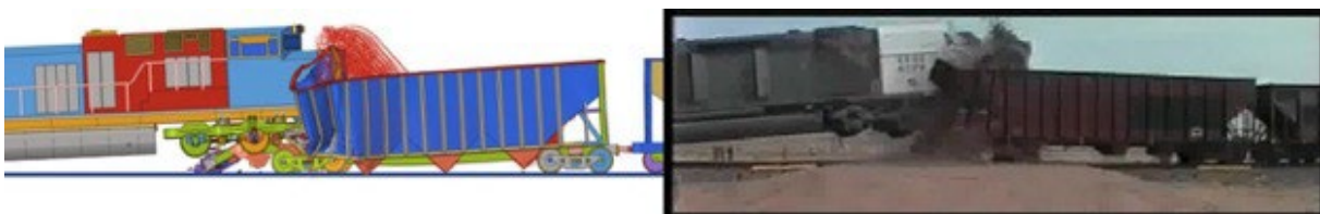
Figure 23. Sequential Images between Simulation and TTC Crash Test at 800 ms
