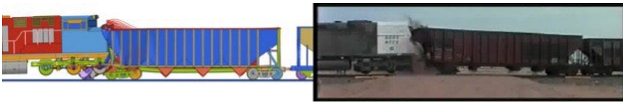
Figure 21. Sequential Images between Simulation and TTC Crash Test at 400 ms
