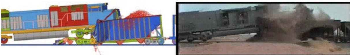
Figure 28. Sequential Images between Simulation and TTC Crash Test at 1,800 ms
