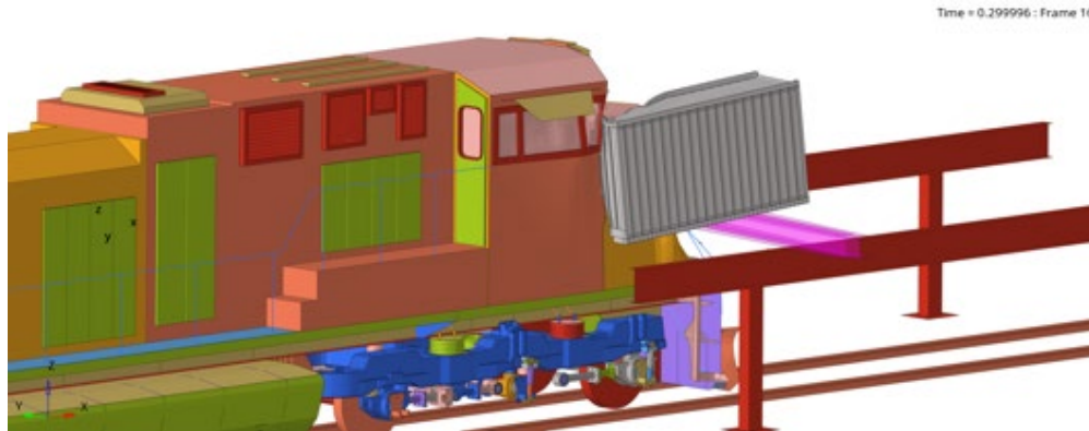
Figure 115. S-580: Rectangular Shape Simulation Sequential Images at 220 ms
