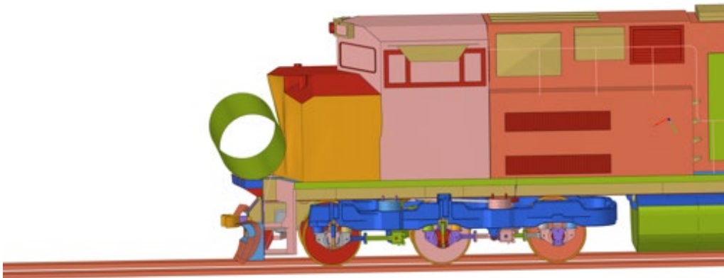
Figure 119. S-580: Cylindrical Shape Simulation Sequential Images for non-modern Locomotive Regulations at 150 ms
