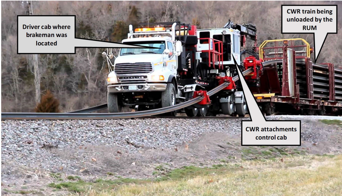
Figure 38. NTSB RAR-21-01 BNSF Railroad Collision Near Kingman, AZ, RUM from CWR Work Train (Source: BNSF)
