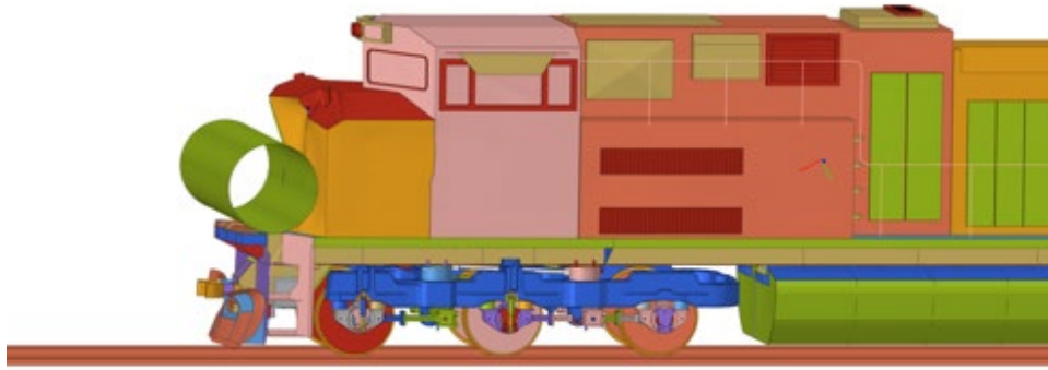
Figure 109. S-580: Cylindrical Shape Simulation Sequential Images at 150 ms
