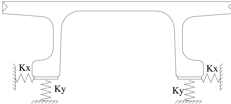
Figure 18. Illustration. Boundary Conditions in the Finite Element Model.
