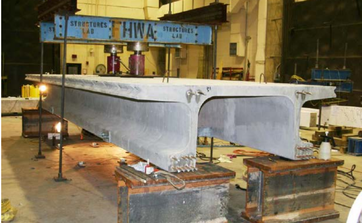
Figure 21. Photo. Test Setup in the Lab.
