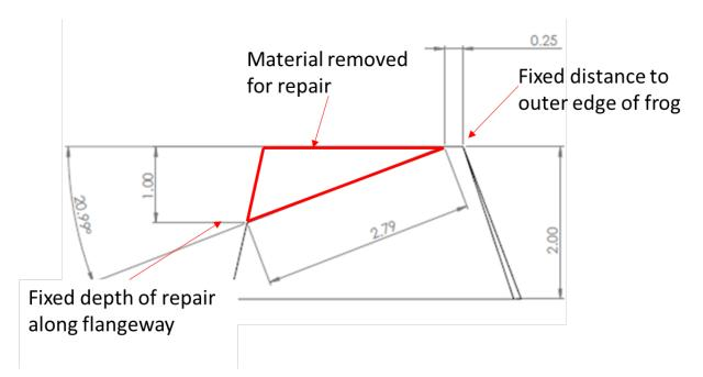
Figure 72. Drawing of a wing cross-section showing material to be replace during an automated repair
