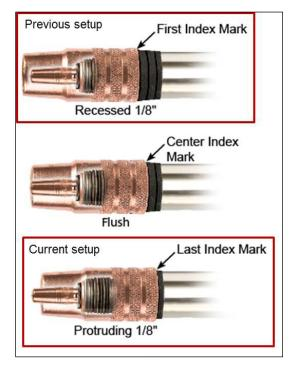
Figure 22. Contact tip position comparison
