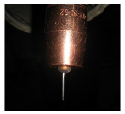
Figure 23. Extended contact tip position
