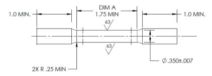
Figure 61. ASTM E8 round tensile dimensions
