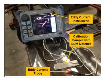
Figure 16. Eddy current equipment setup
