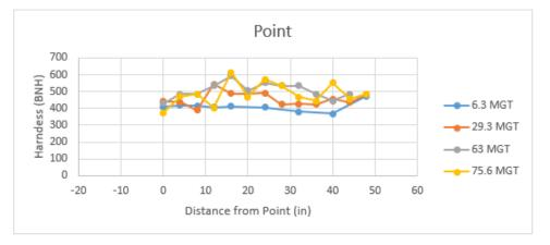
Figure 99. Hardness measurements: NS frog, point
