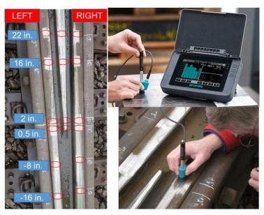
Figure 40. Hardness measurements in each of the red oval locations: Proceq hardness tester (top-right) and measurements from the CSX frog (bottom-right)
