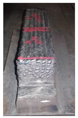
Figure 3. Buildup marked for testing
