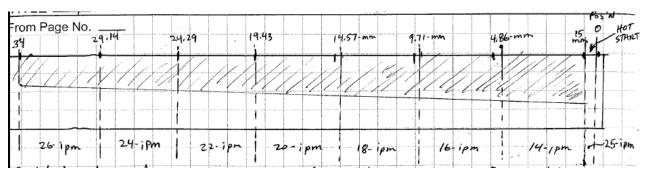
Figure 74. Travel speed segments for tapered wing welding
