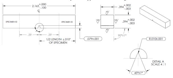
Figure 62. ASTM E23 CVN specimen dimensions
