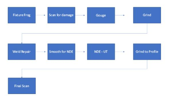
Figure A-1. Automated repair process flow diagram
