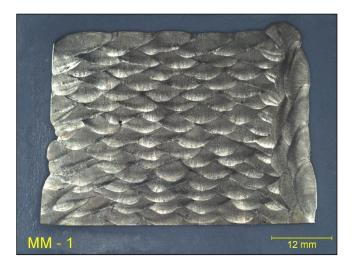
Figure 10. Metal-cored wire macrograph (CV parameters)
