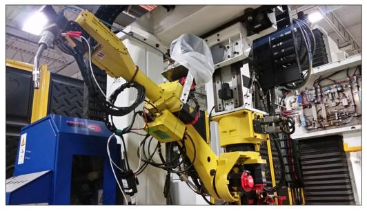
Figure 84. Fanuc robotic welding system used for automate weld repair
