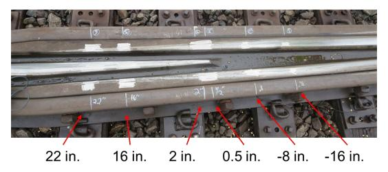
Figure 37. Profile measurement locations on the frog
