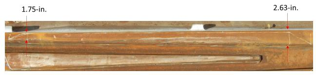
Figure 71. WBM varying wing width along the repair area
