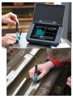
Figure 96. Proceq hardness tester (top) and measurements being taken on a repaired frog (bottom)
