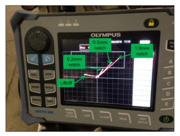
Figure 17. Eddy current response from calibration notches
