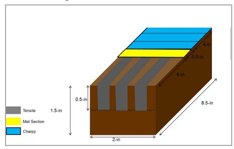
Figure 7. Weld buildup test specimen locations
