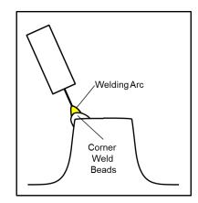
Figure 85. Corner/edge bead welding
