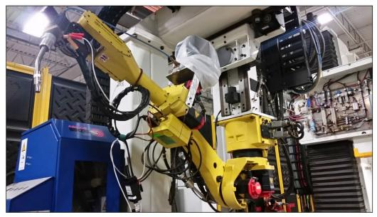
Figure 18. Fanuc robot utilized for welding
