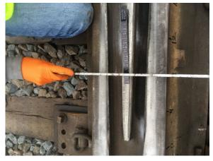
Figure 94. Wear measurements being taken with a straightedge and taper gauge
