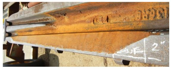
Figure 76. Practice rail-bound frog with simulated WBM wing repair cut
