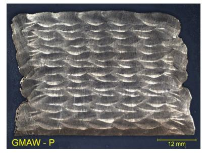
Figure 11. Metal-cored electrode macrograph (GMAW-P)
