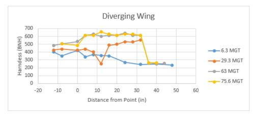
Figure 98. Hardness measurements: NS frog, diverging wing
