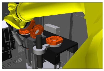
Figure A-12. Robot with tool changer approaching tool for connection
