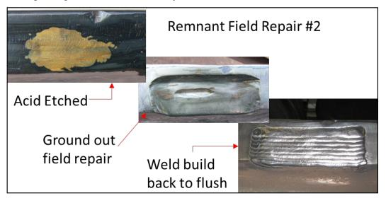
Figure 82. Example of field repair removal and automated weld repair buildup
