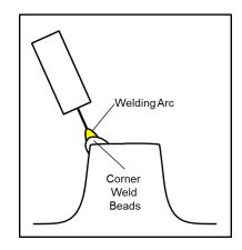
Figure 4. Corner/edge bead welding
