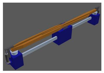
Figure A-2. Part clamping fixture
