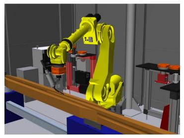
Figure A-8. Robot with welding torch
