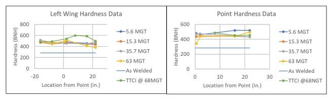
Figure 48. Comparison plot of hardness measurements
