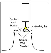
Figure 5. Center bead welding
