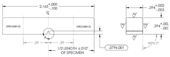
Figure 9. CVN specimen configuration
