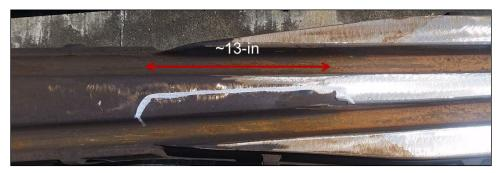
Figure 33. Area on point, outside of repaired area, with uneven deformation
