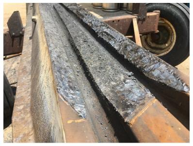
Figure A-4. Example of frog after damaged rail section removed
