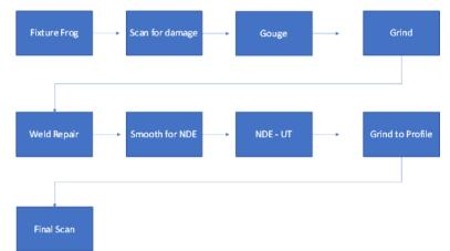
Figure 101. Fully automated frog repair process flow diagram
