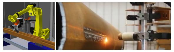
Figure A-5. Robotic plasma gouging
