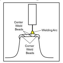
Figure 86. Center bead welding
