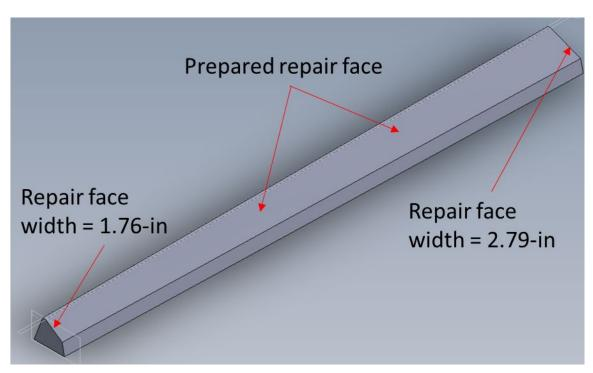
Figure 73. Model of a WBM wing prepared for automated repair
