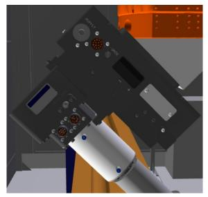
Figure A- 18. Servo spindle and compliance device
