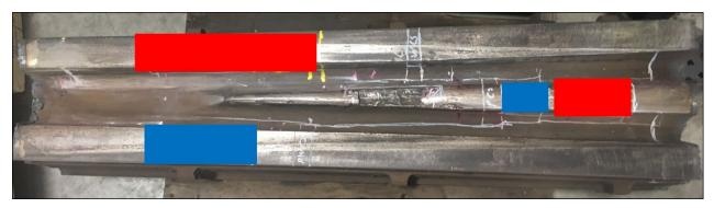
Figure 60. Mechanical test specimen cut plan, tensile bars from red areas, and CVN specimens from blue areas
