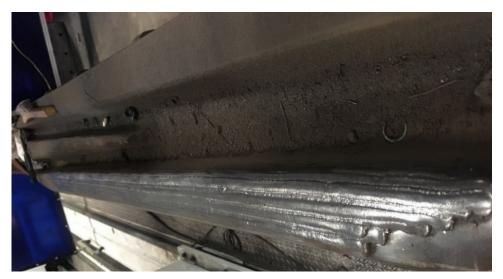
Figure 77. Practice rail bound frog with automated weld repair
