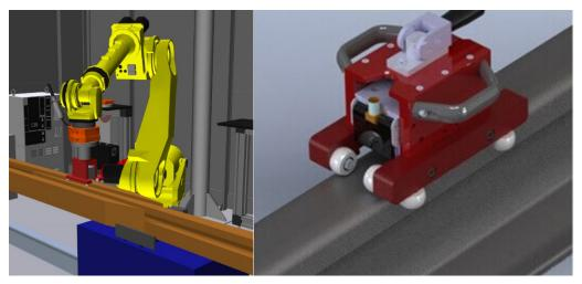
Figure A-7. EMAT sensor carried by robot (left) and manual EMAT sensor (right)
