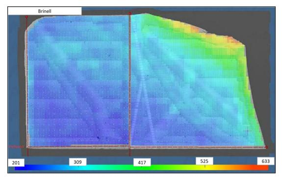
Figure 51. Right wing cross-section with hardness map
