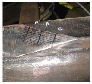
Figure 83. Map of hardness measurements taken on the point joint face
