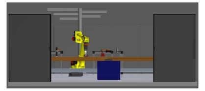
Figure A-14. Tool bundle tree shown behind robot
