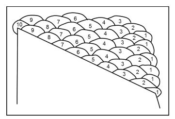
Figure 26. CSX frog wing repair welding sequence
