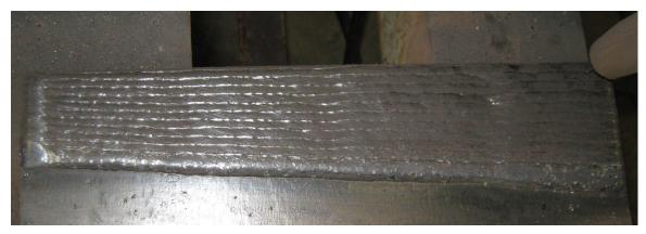
Figure 75. Tapered bead test plate with varied travel speed to narrow build area
