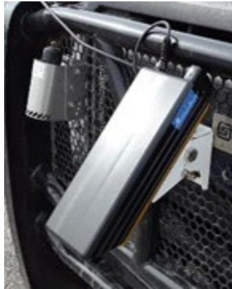
Figure 6.3: Mobile IceSight mounted on the front of an Abilene District pickup truck
