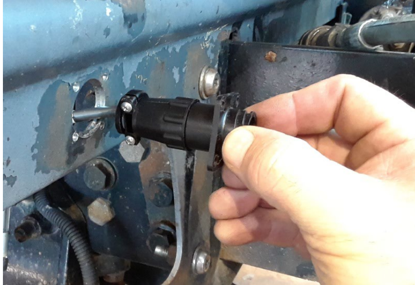
Figure 3.8: A hole is drilled on the bumper to install the cable plug assembly.
