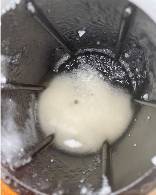
Figure 5. Truck filter clogged with solid salt crystals.
