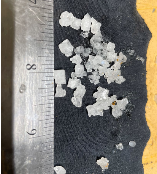
Figure 4. Presumed rock salt crystals, found in the screen filter from the liquid application system.
