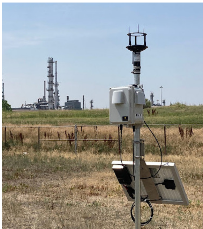
A 2B Tech AQ Sync Monitor is pictured at its installed location, I-270 and York Street. Credit: Photo Courtesy of the Colorado Department of Transportation (Steve Cohn, Environmental Programs Branch)
