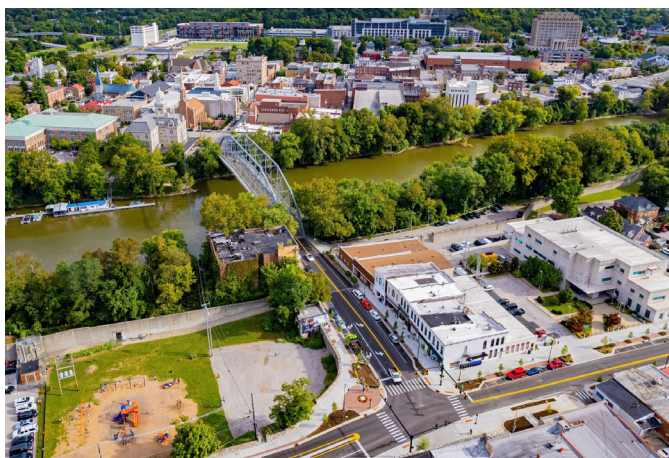
Intersection modifications improved mobility for vulnerable users. At the intersection of Bridge Street and Second Street, the crossing distance was cut in half, free flow turn movement conflicts with pedestrians were eliminated, and pedestrian signal enhancements were implemented. Credit: Photo Courtesy of Strand Associates, Inc. and Abstract Photography, Inc.
