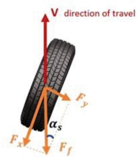
Figure 6.12 Top view of the tire under pure sideslip cornering conditions.
