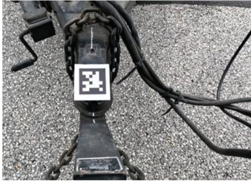
Figure 5.5 Calibrated video frame at zero articulation angle.
