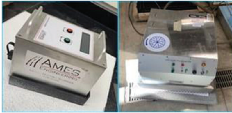
Figure 2.3 Texture measuring devices (left: LTS; right: CTM).
