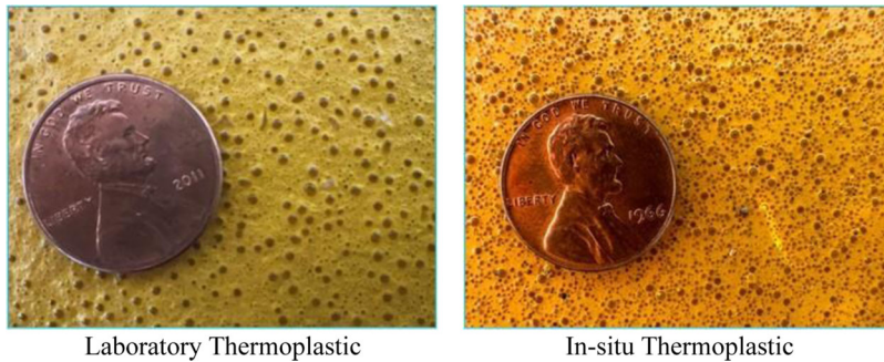
Figure 2.22 Closeups of thermoplastics applied in laboratory and in field.
