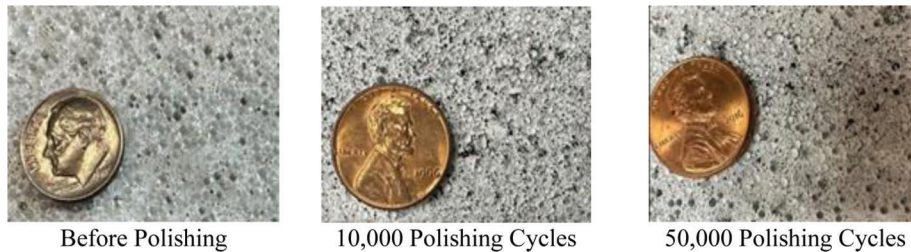
Figure 2.13 Polyurea specimen surface during polishing.
