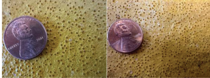
Group 16-Thermoplastic (left: before polishing; right: after 100,000 polishing cycles)
