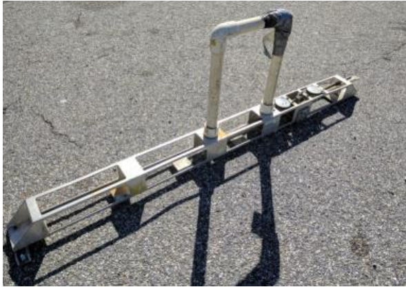
Figure 16. ALDOT Beam (Left) and Inertial Profiler (R) (Giler, 2017)
