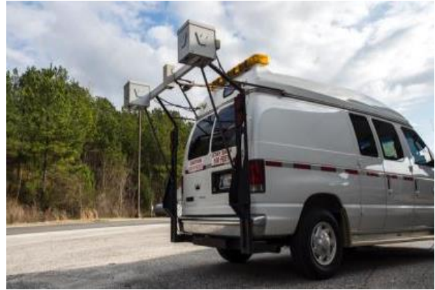
Figure 16. ALDOT Beam (Left) and Inertial Profiler (R) (Giler, 2017)
