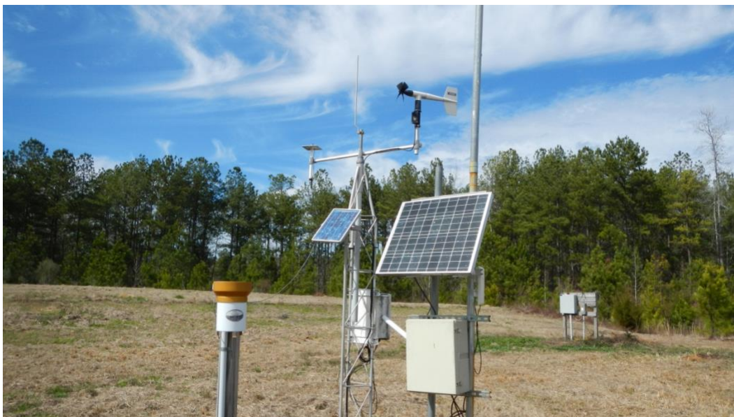
Figure 15. Weather Station at NCAT Test Track
